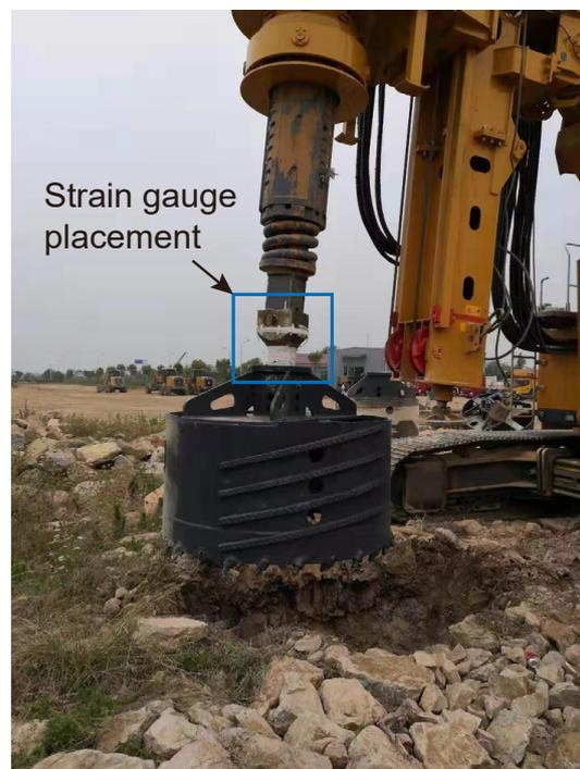
**Figure 4.** Load testing of drill pipe on rotary drilling rig.
