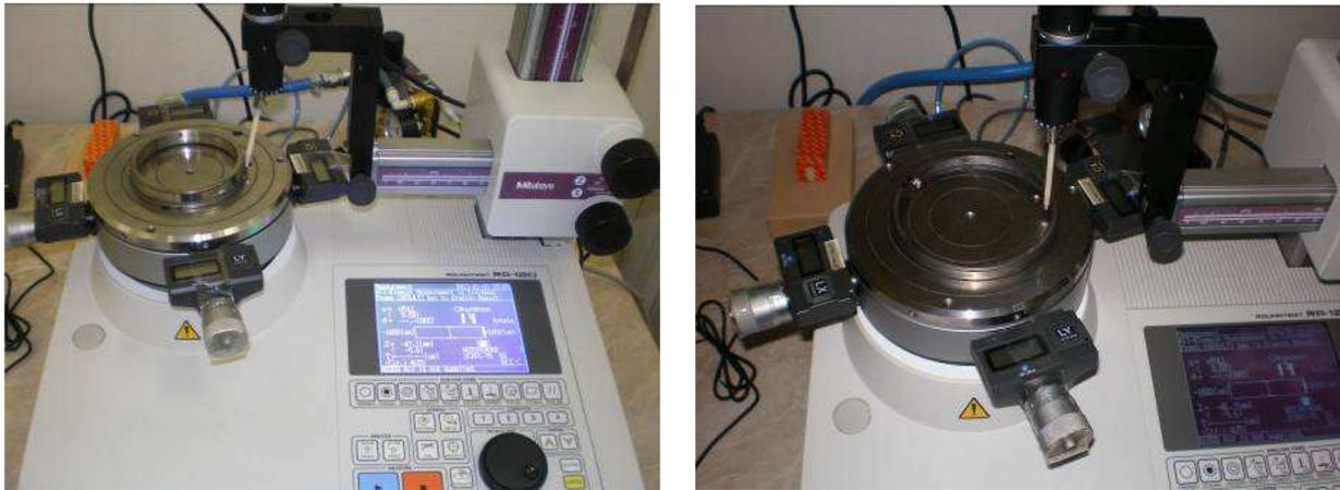
Figure 9. Measurement of circularity on the orbits of the inner and outer rings of bearing 31312.
