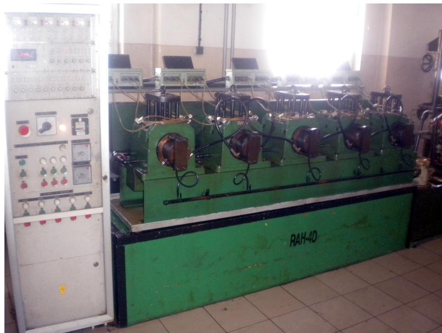
**Figure 7.** Testing station for bearing diagnostics RAH-4D with unmanned operation.
