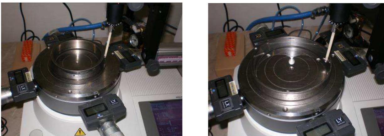
**Figure 10.** Measurement of circularity on the orbits of the inner and outer rings of bearing 32314.
