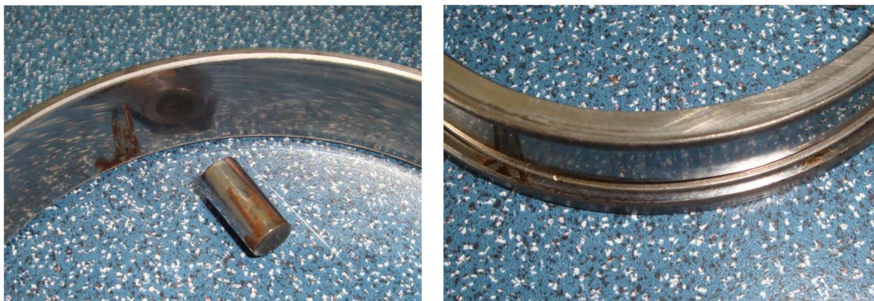
**Figure 6.** Local surface corrosion on both the rolling body shell and the outer orbit ring.
