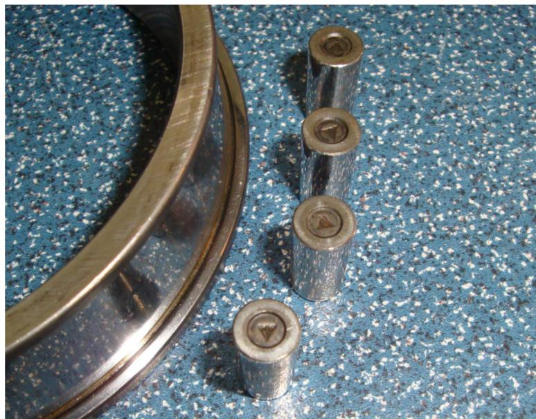
**Figure 5.** Condition of the rolling elements and inner ring of the bearing under consideration after disassembly.
