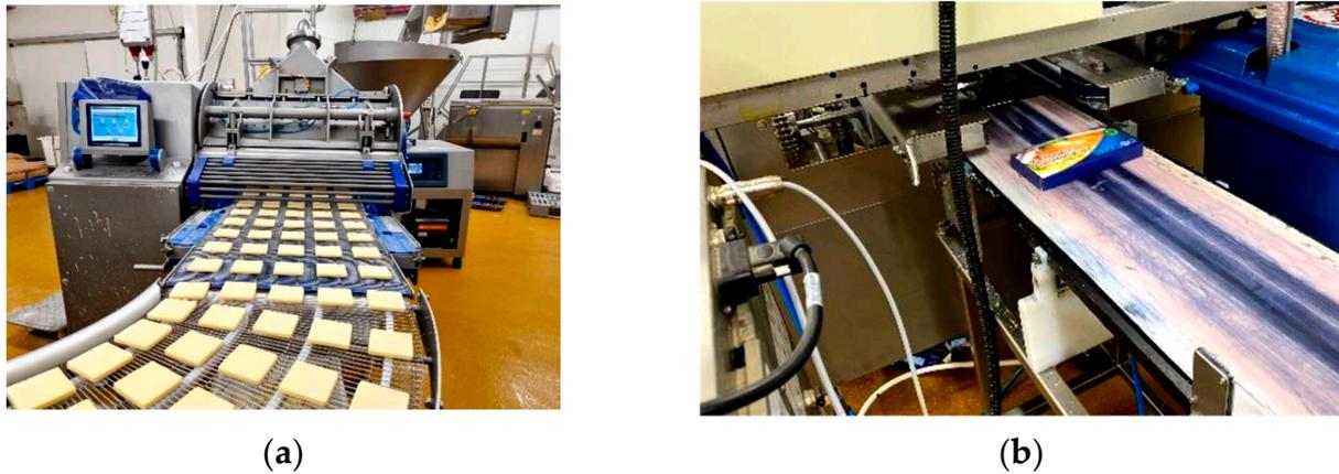
**Figure 8.** Merrell forming machine and Econopack packer [21]. (a) Merrell forming machine; (b) Econopack packer.
