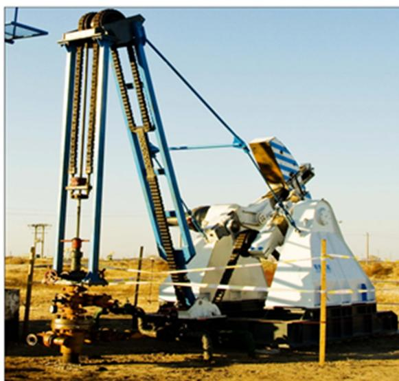
Figure 20. Photo of eccentric flexible pumping unit in oil field application.
