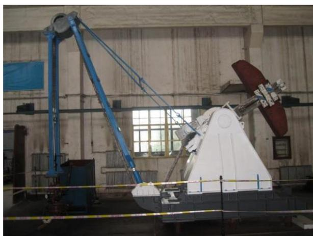
**Figure 18.** Indoor test photos of eccentric balanced pumping unit.
