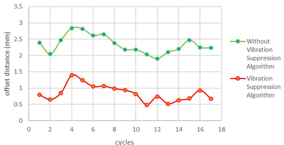
Figure 11. Joint vibration suppression at 150% of straightness velocity.
