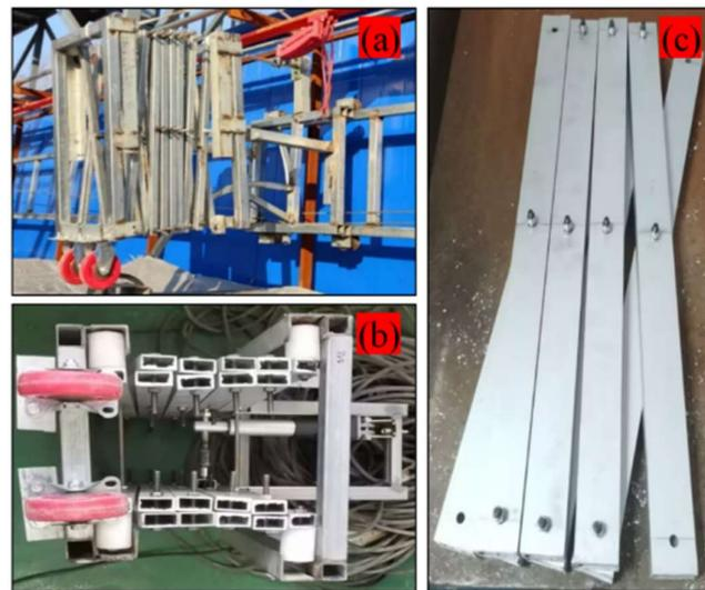
**Figure 14.** (a) Prototype running test; the scissor arm is made of a square tube. (b) Second prototype running test; the scissor arm is made of aluminium profile. (c) The scissor arm connection hole is deformed and badly worn.
