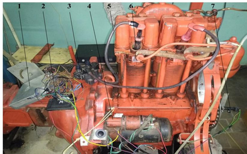
**Figure 5.** Ignition system of the experimental diesel/hydrogen mixture engine D21: 1—control unit; 2—ignition amplifier; 3—ignition DIS-module; 4—starter of engine; 5—spark wires; 6—high-voltage plugs; 7—sensor of crankshaft.
