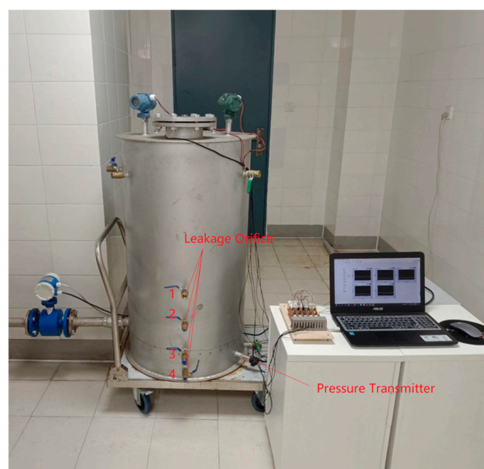
Figure 7. Orifice leakage simulation platform for storage tanks.
