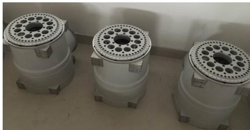
**Figure 11.** Mock-up of joints after mass-matching.
