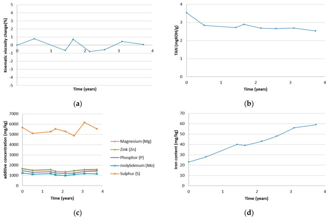
**Figure 6.** Sampling results of PAO II during the period of analysis. (a) Changes in the kinematic viscosity; (b) TAN; (c) additive content measured by the ICP method; (d) iron content measured by the ICP method.
