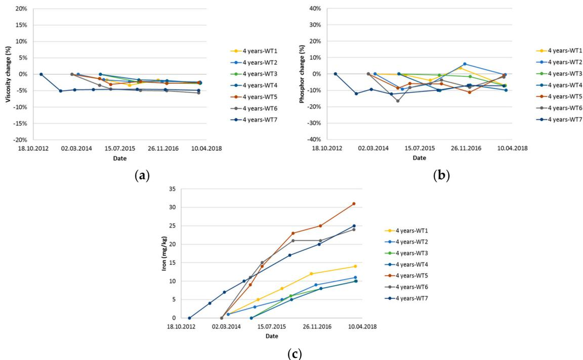
**Figure 8.** Trend analysis for the four-year turbine group with PAO I. (a) Changes in the kinematic viscosity; (b) changes in the phosphorus content measured by the ICP method; (c) iron content measured by the ICP method.
