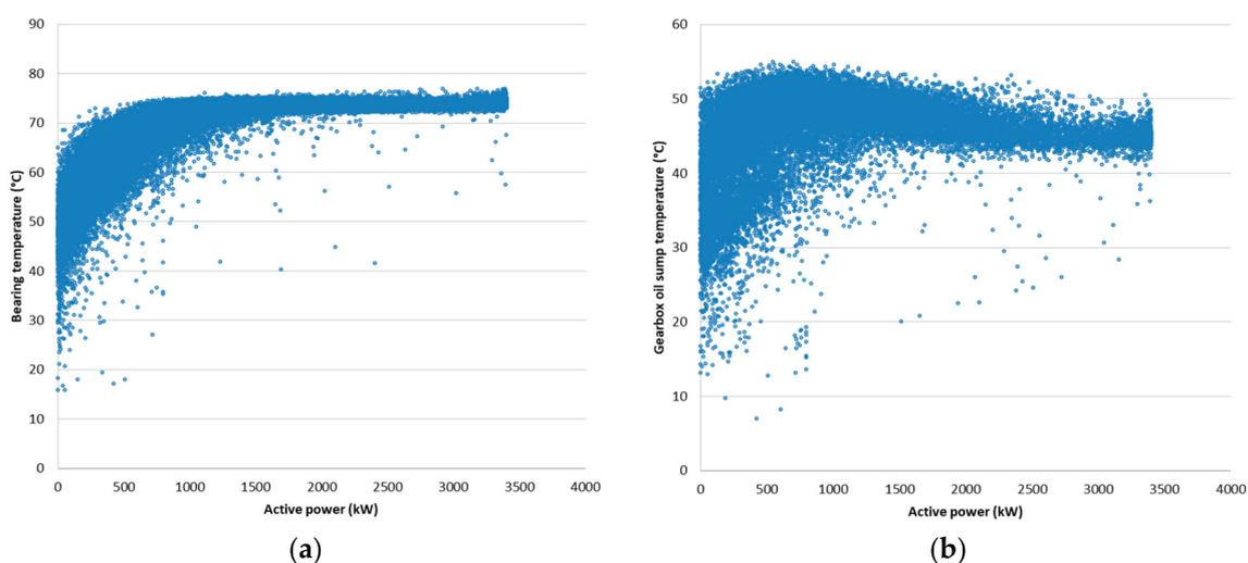
**Figure 7.** Gearbox temperature power functions during the first oil sampling interval of approx. six months. (a) Bearing temperature as a function of the active power ( $P_{\text{act}} > 0$ ); (b) gearbox oil sump temperature as a function of the active power ( $P_{\text{act}} > 0$ ).
