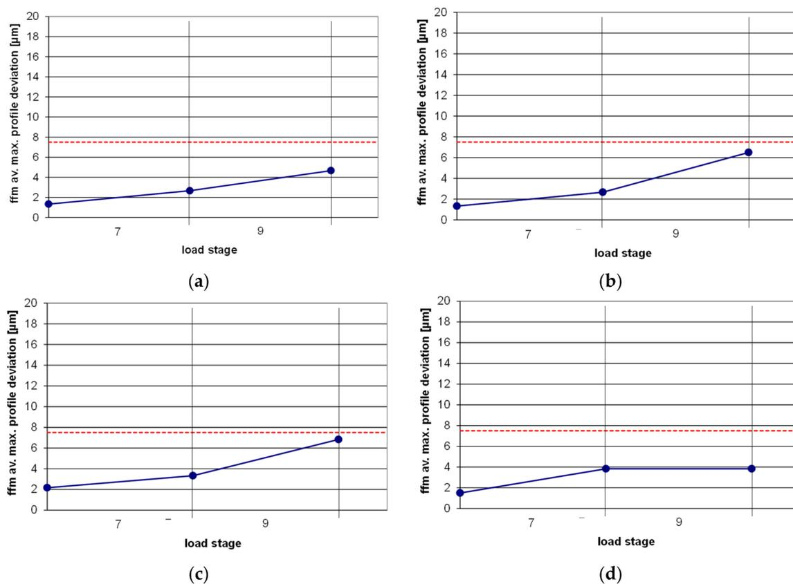
**Figure 4.** Micropitting test results for PAO: (a) fresh oil; (b) oil aging stage I; (c) oil aging stage II; (d) oil from the field.
