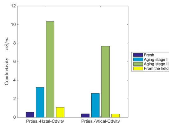
**Figure 3.** Conductivity measurements of fresh and aged mineral oil.
