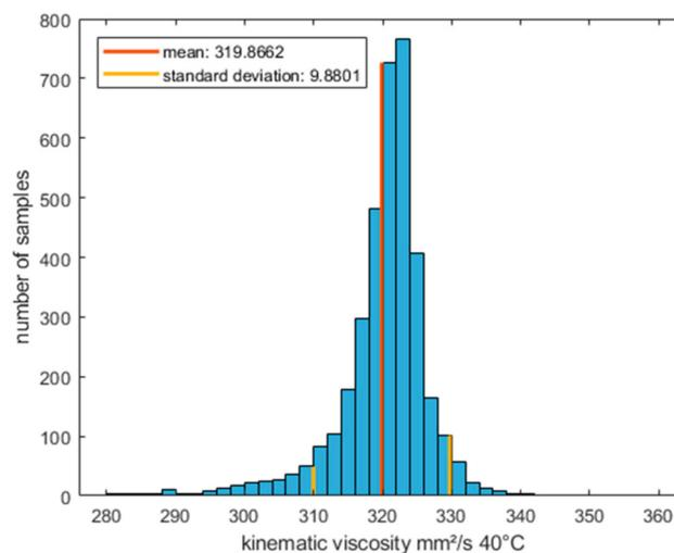
**Figure 10.** Distribution of the kinematic viscosity at 40 °C of PAO III.
