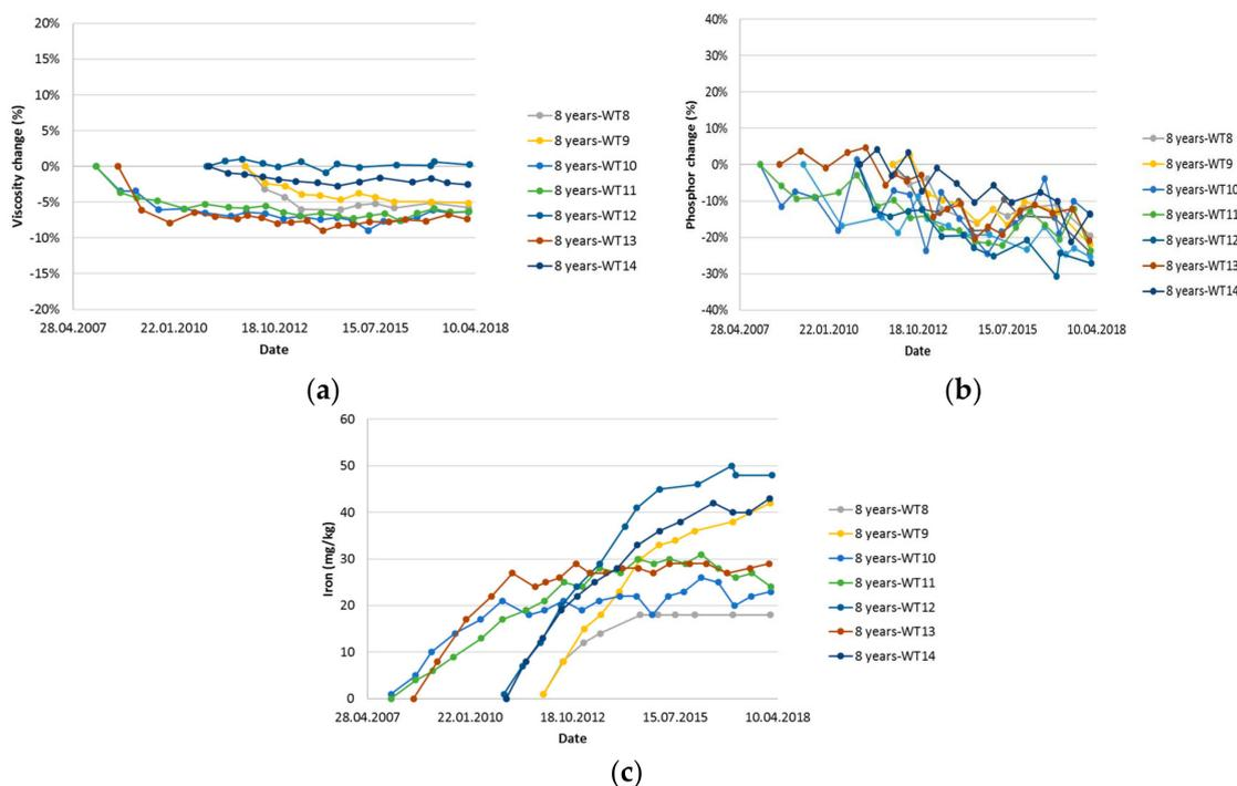
**Figure 9.** Trend analysis for the eight-year turbine group with PAO I. (a) Changes in the kinematic viscosity; (b) changes in the phosphorus content measured by the ICP method; (c) iron content measured by the ICP method.
