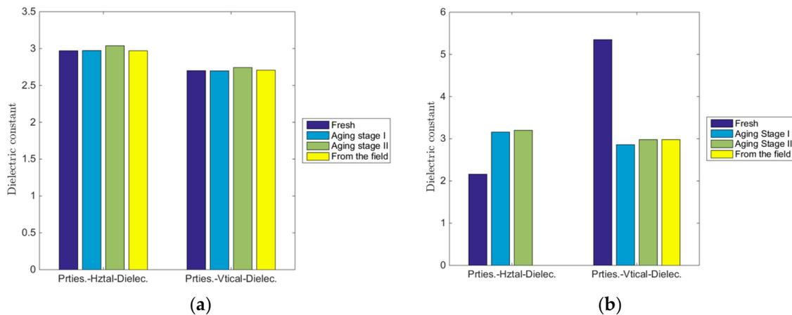
**Figure 2.** Measured dielectric constant of (a) mineral oil and (b) PAG oil during the stepped profile described in Section 3.2.2.
