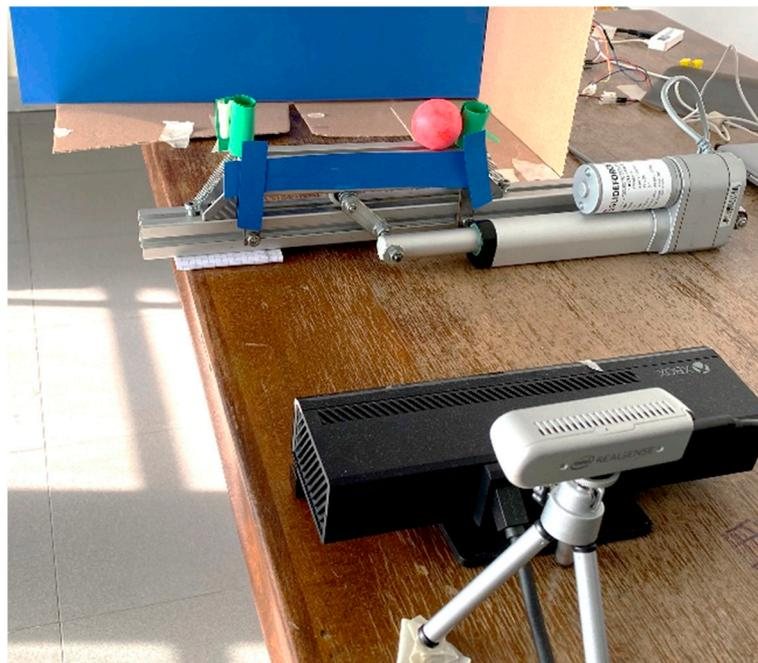
Figure 11. Experimental apparatus with a slide moved by the linear actuator for the ball equilibrium application.
