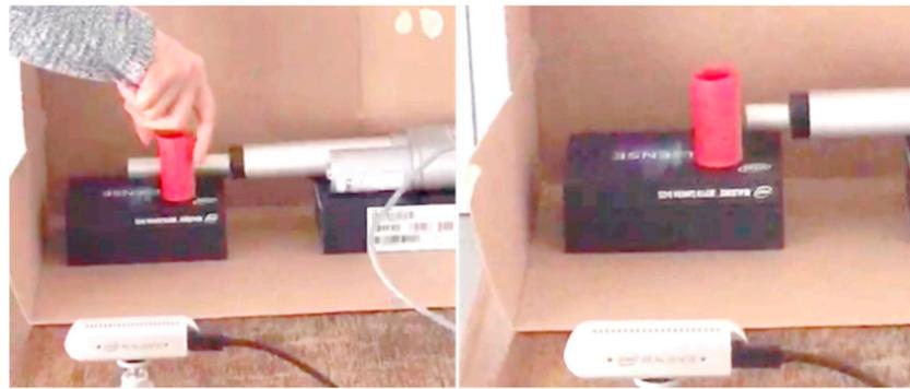
**Figure 8.** The actuator tracks the target object even if the target is placed behind the actuator (Left, Right).
