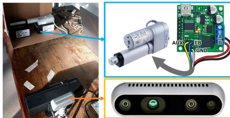
**Figure 1.** Test bench adopted for measurement: linear actuator, board control and 3D acquisition camera.
