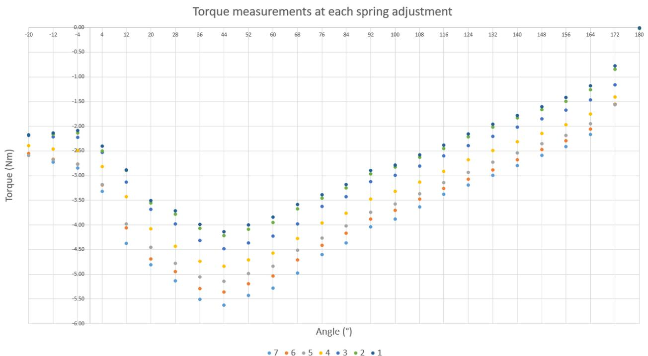
**Figure 8.** Computed static torques with the testbench configuration (at one extreme of the shoulder translation joint) for each of the seven spring levels in MATE. Level 7 is the strongest one, and level 1 is the weakest.
