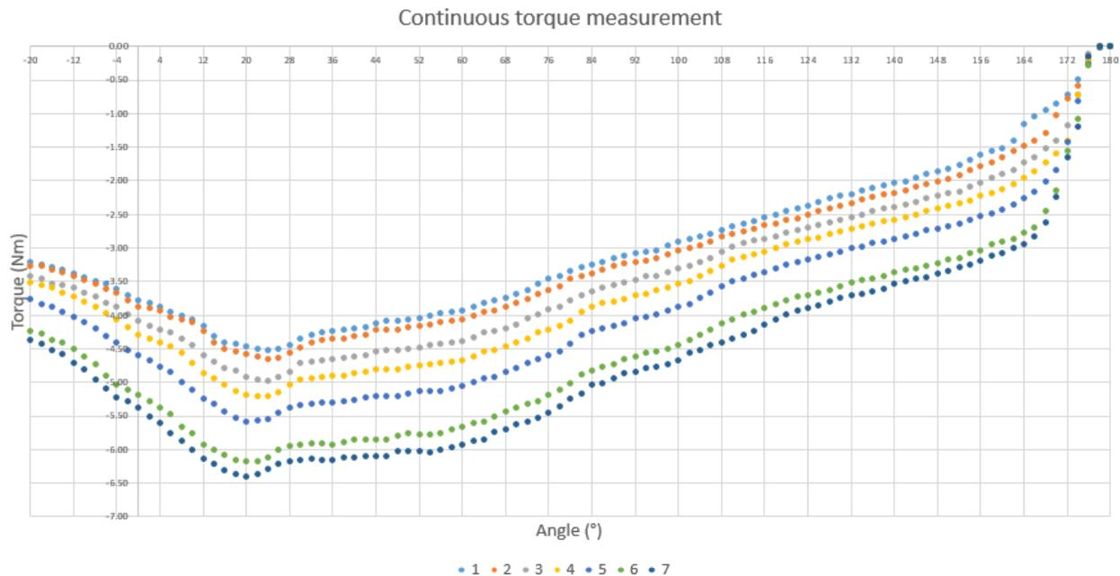
**Figure 9.** Computed dynamic torques with the testbench configuration (at one extreme of the shoulder translation joint) for each of the seven spring levels in MATE. Level 7 is the strongest one, and level 1 is the weakest.
