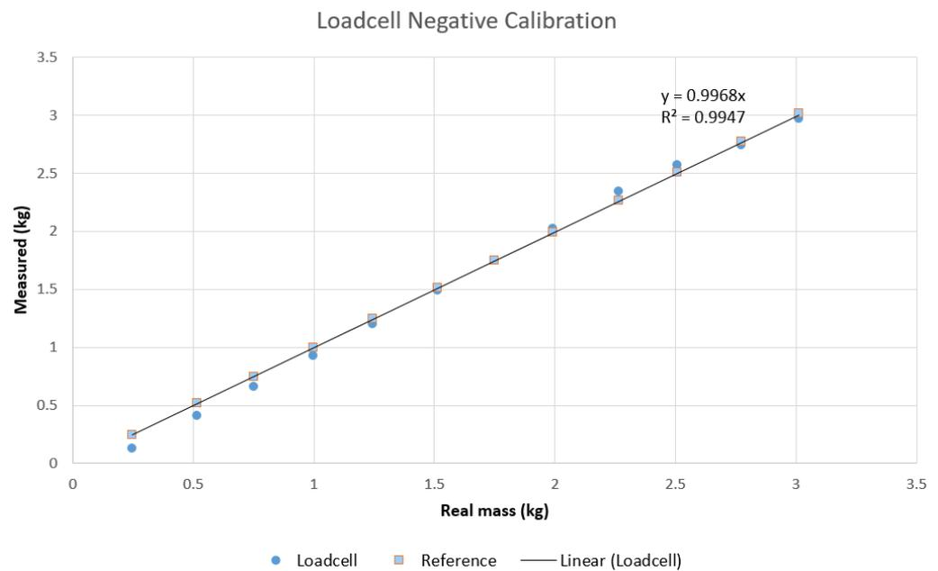
**Figure 4.** Beam load cell negative linearity.
