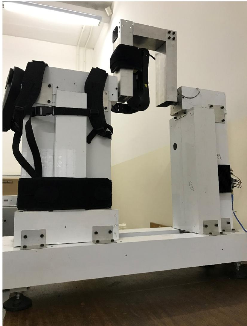
**Figure 1.** Exoskeleton mounted on the test bench.
