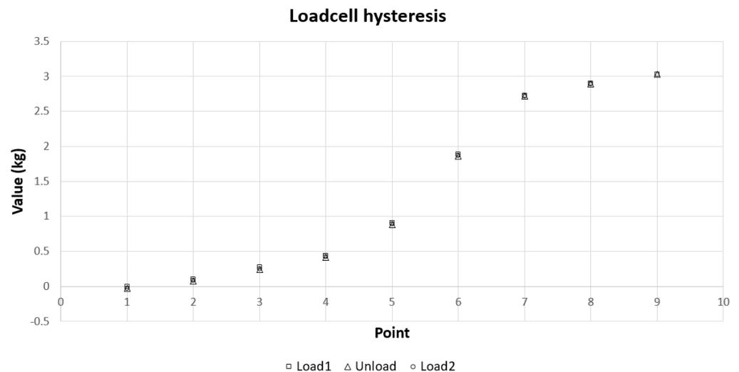
**Figure 5.** Beam load cell hysteresis behavior.
