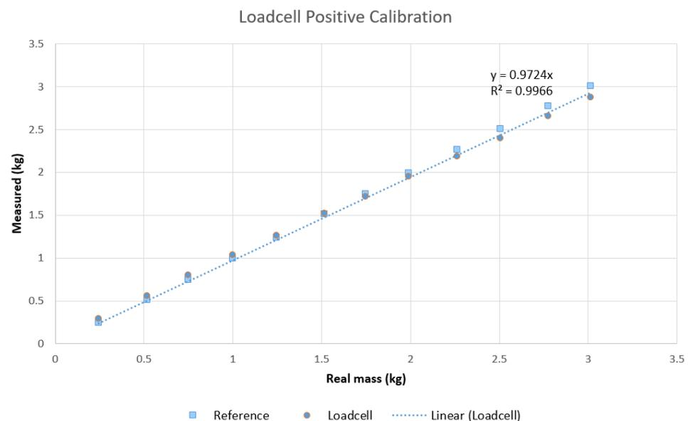
**Figure 3.** Beam load cell positive linearity.
