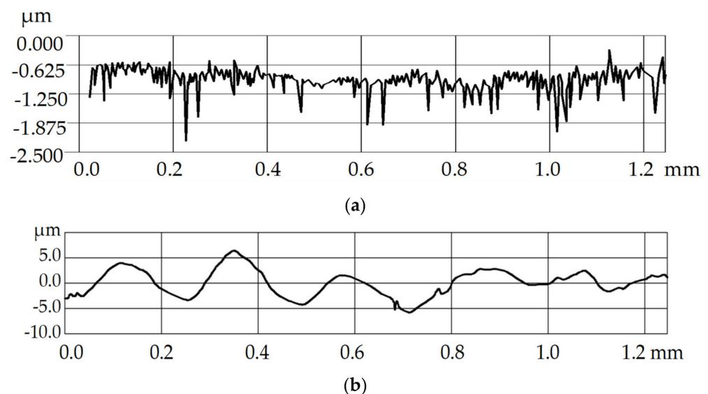
**Figure 6.** Profilograms of the test specimen surface: (a)-after rolling; (b)-after fine turning, with the formation of a regular microrelief.
