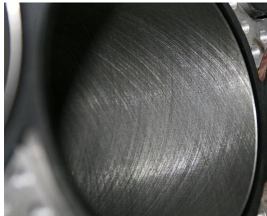
**Figure 1.** The surface structure of the cylinder liner of the internal combustion engine formed by honing [20].
