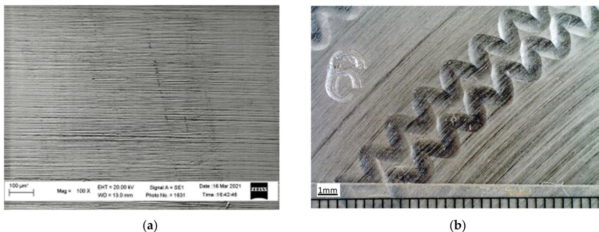
Figure 5. Photographs of specimen surfaces from steel 17G1S during finishing operations of the technological process: (a) after rolling; (b) ball burnishing, with the formation of a regular microrelief.
