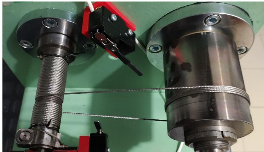
Figure 16. Cable-driven transmission 25–75 G.
