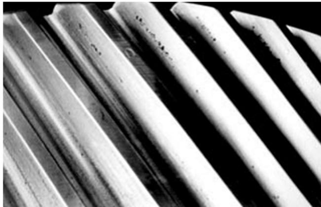
**Figure 5.** The initial pitting in the connection stage of a pair of teeth—1. Reprinted with permission from ref. [24]. Copyright 2003 Springer
