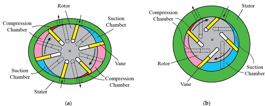
**Figure 1.** Sliding vane compressor schematics and operating principle: (a) elliptical stator with radial vanes; (b) cylindrical stator with canted vanes.
