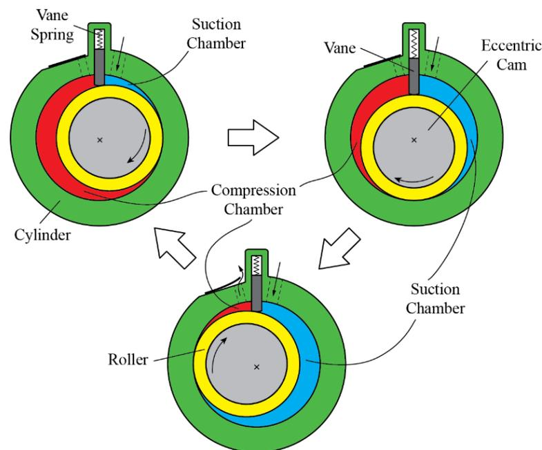
**Figure 3.** Rolling piston compressor working principle.
