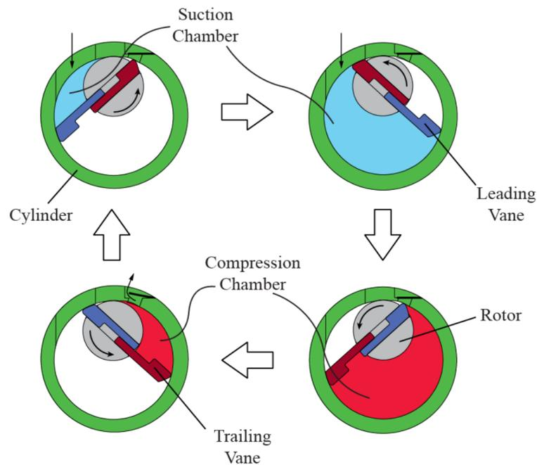
**Figure 2.** Coupled vane compressor working principle.
