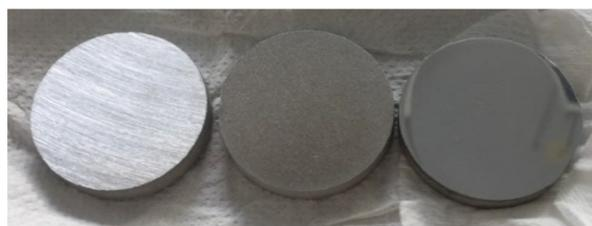
**Figure 3.** From left to right: example of S235 samples, scratched, sanded, and mirror-polished, respectively.
