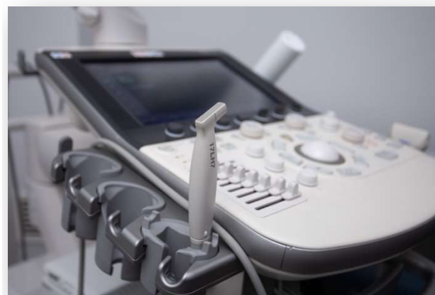
Figure 3. A high-frequency 'hockey stick' linear transducer.
