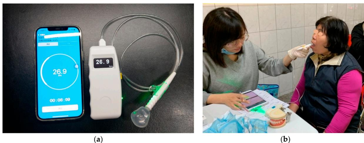
**Figure 1.** (a) A tongue pressure measurement device with wireless mobile application control function and a disposable oral positioning mouthpiece. (b) The tongue pressure device and its usage in the measurement of tongue pressure.
