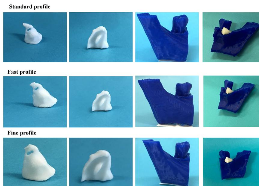
**Figure 30.** Images of the FDM 3D-printed scaffolds for Patient 3, produced using the three different printing profiles (left to right: scaffold 1, scaffold 2, the alveolar bone, and the scaffolds applied to the periodontal defect.).
