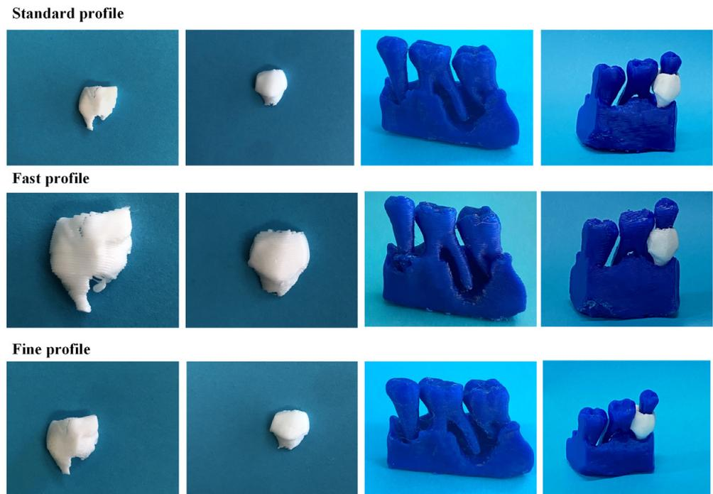
**Figure 10.** Images of the FDM 3D-printed scaffolds for Patient 1, produced using the three different printing profiles (from left to right: scaffold 1, scaffold 2, alveolar bone, and scaffolds applied to the periodontal defect).
