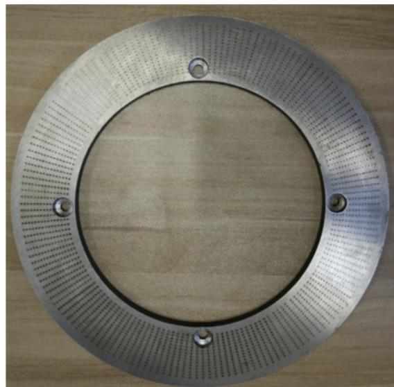
**Figure 18.** Surface texture of separator disk.
