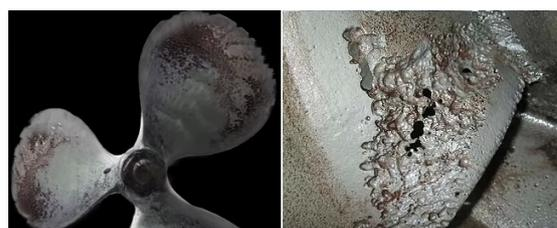
**Figure 1.** Cavitation damage on propeller.
