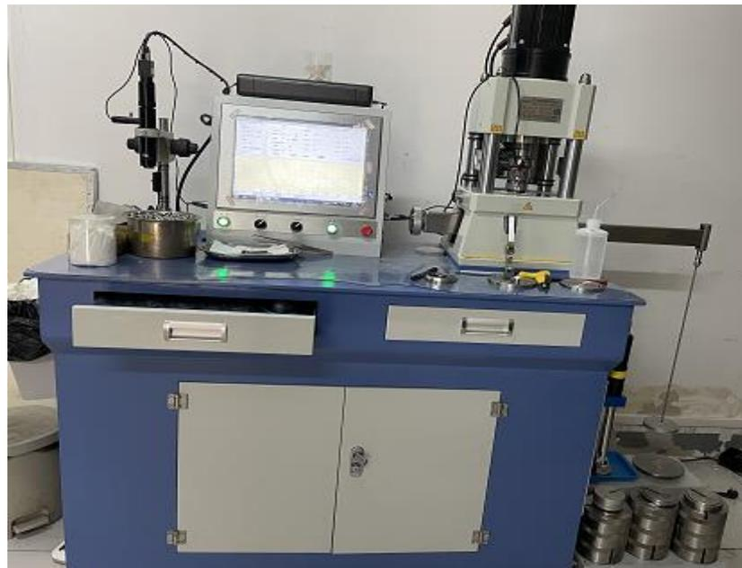
**Figure 1.** The real images of four-ball tribometer used.
