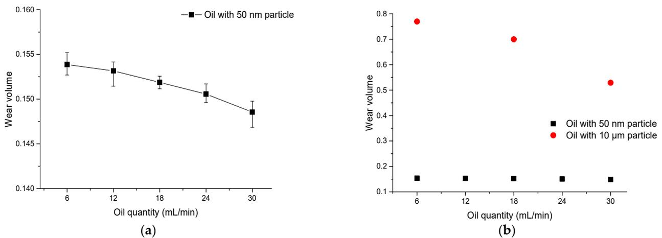
**Figure 6.** Variation law of wear under different oil quantity: (a) wear volume of the complete embedded under various oil supply; (b) comparison of wear volume under different embedded conditions.
