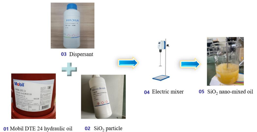
**Figure 1.** Preparation process of nano-mixed oil.
