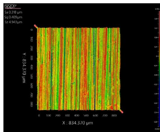
**Figure 3.** Surface microtopography of the roller bearing.
