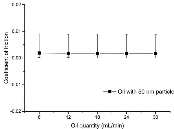
**Figure 5.** Variation law of coefficient of friction under different oil quantities.
