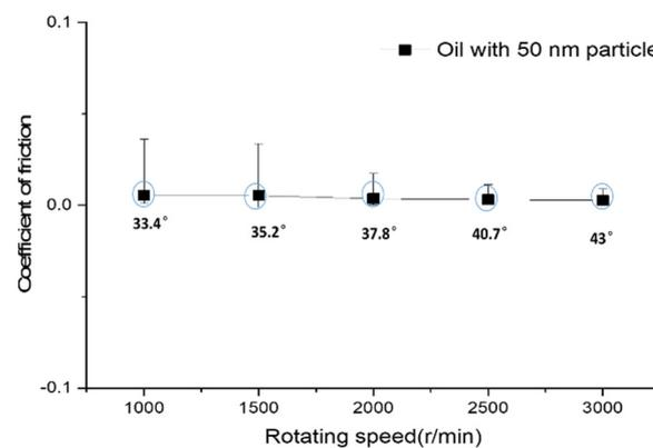
Figure 7. Variation law of coefficient of friction under different speeds.
