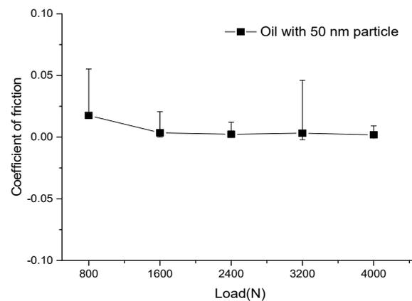
Figure 9. Variation law of coefficient of friction under different loads.
