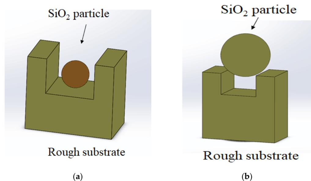
**Figure 4.** Embedding conditions: (a) complete embedded case; (b) complete non-embedded case.
