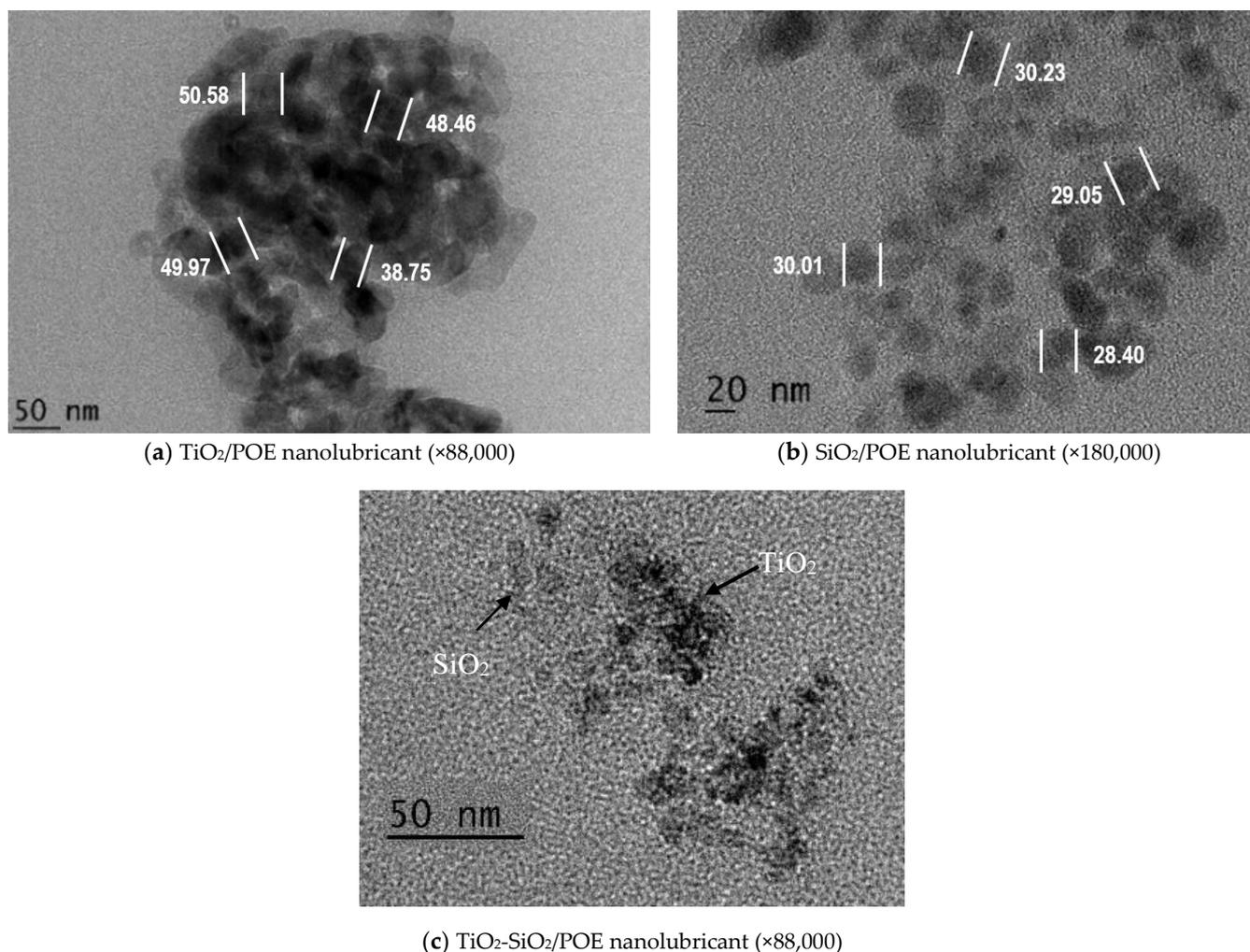
**Figure 5.** TEM images for mono and hybrid nanolubricants.
