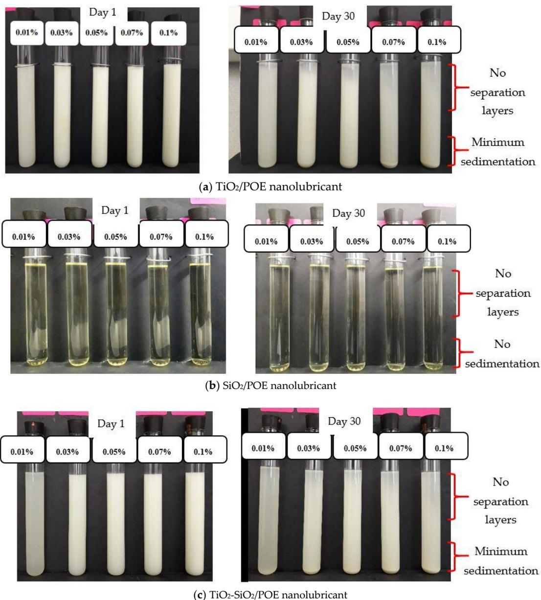
**Figure 3.** Nanolubricants sedimentation observation for up to 30 days after preparation.
