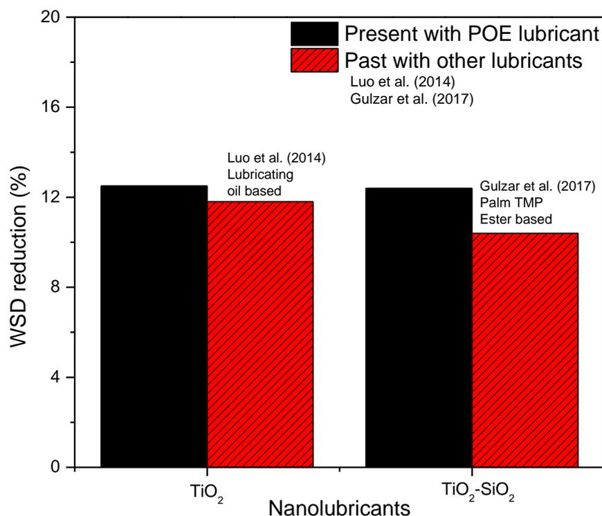
**Figure 10.** Wear scar diameter reduction comparison with previous studies.
