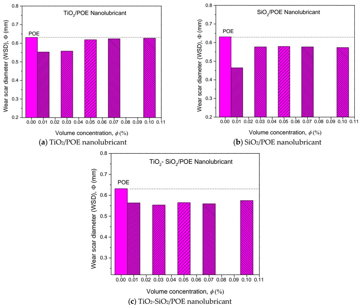
**Figure 9.** Wear scar diameter for mono and hybrid nanolubricants.
