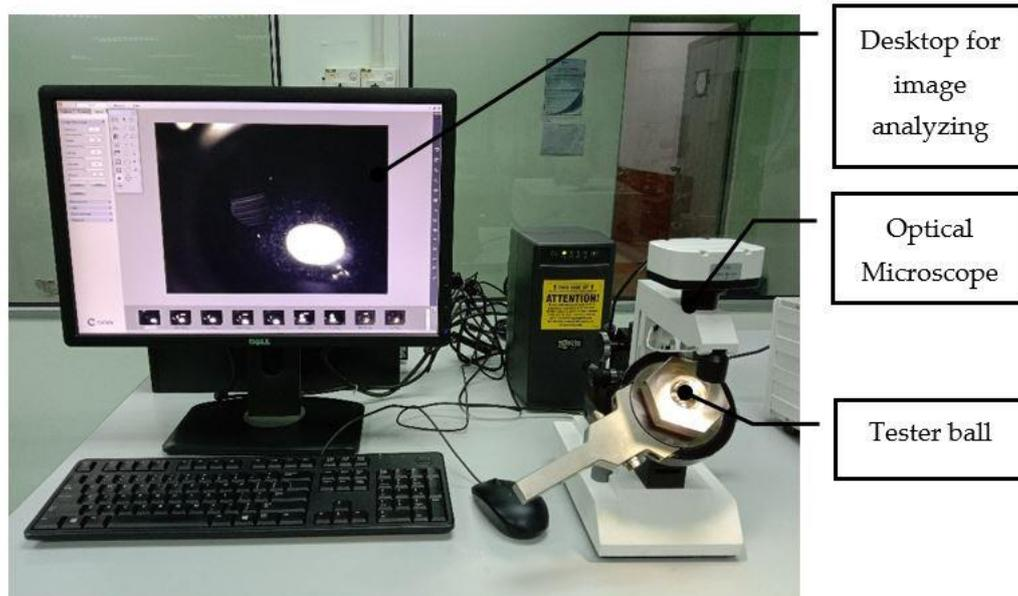
(b) Wear scar diameter microscope
