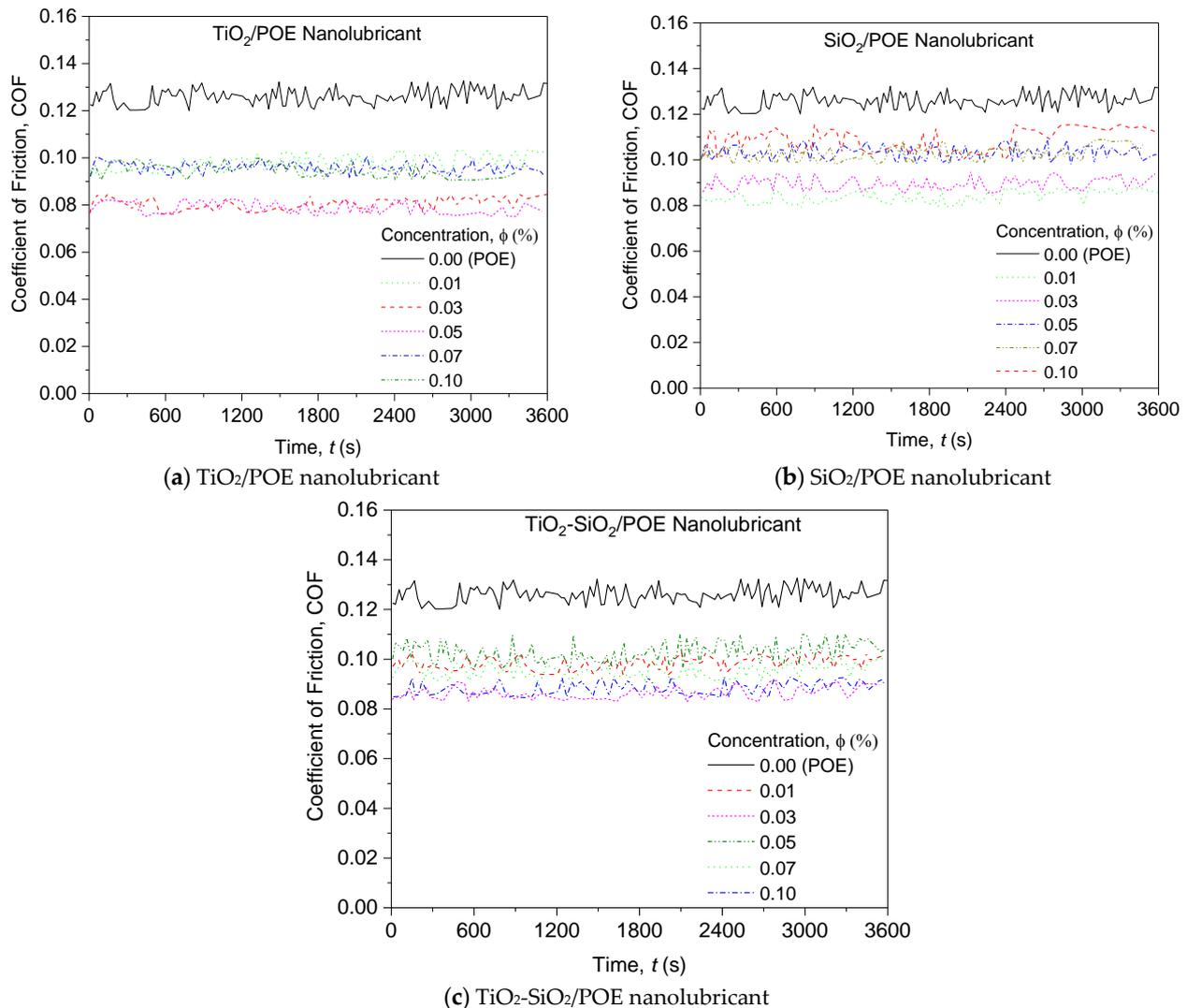
**Figure 7.** Coefficient of friction for mono and hybrid nanolubricants.
