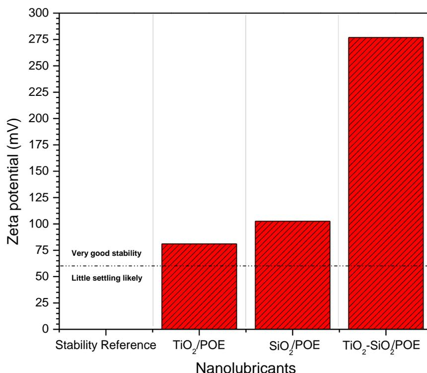
**Figure 4.** Zeta potential of  $\text{TiO}_2/\text{POE}$ ,  $\text{SiO}_2/\text{POE}$  and  $\text{TiO}_2\text{-SiO}_2/\text{POE}$  nanolubricants.
