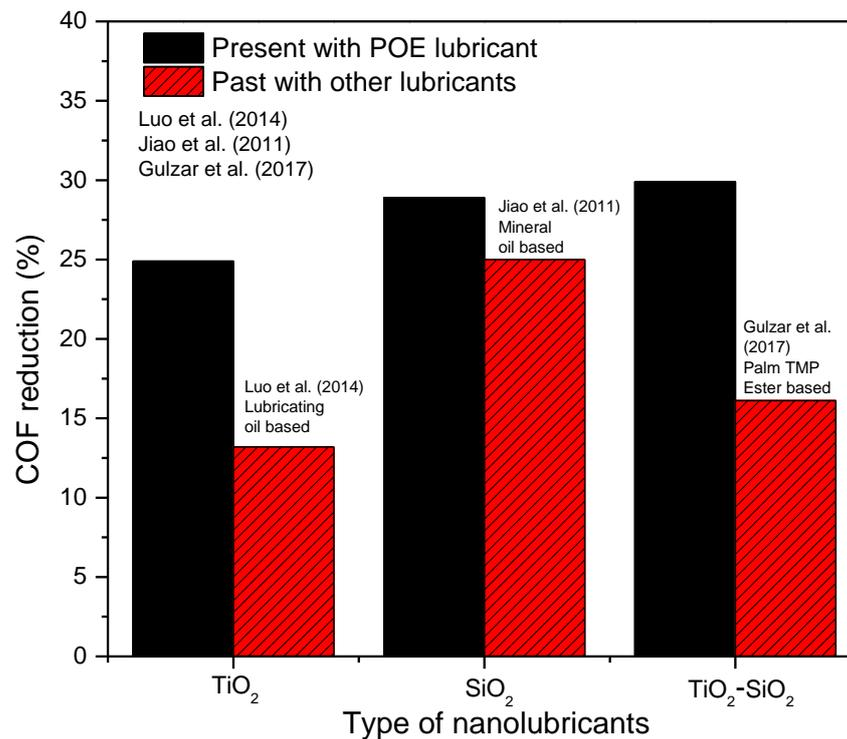
**Figure 8.** Comparison of coefficient of friction reduction with previous studies.
