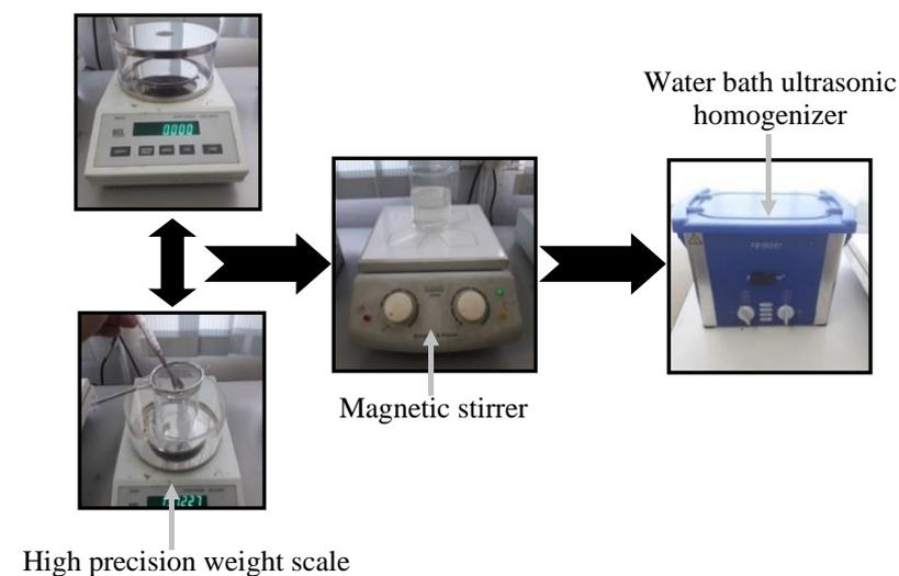
**Figure 1.** Two-step process in preparation of the nanolubricants.
