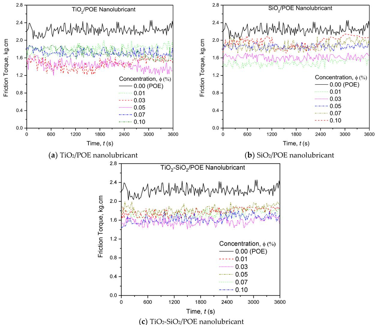
**Figure 6.** Friction torque for mono and hybrid nanolubricants.
