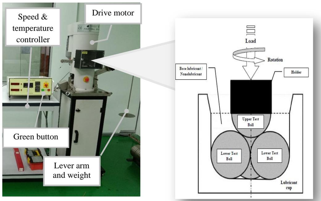
(a) Four-Ball tribology tester and its schematic configuration
