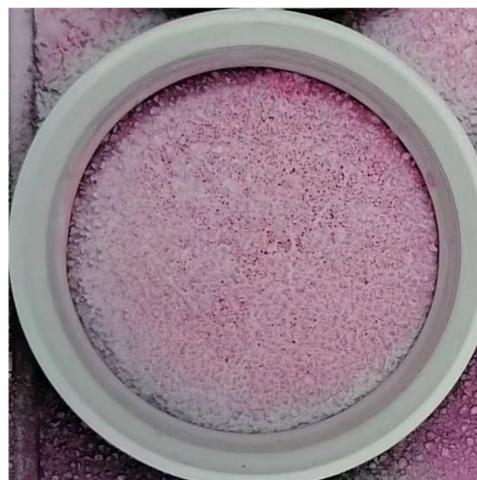
**Figure 8.** Phosphor flaw-detection results of the laser-melting valve seat.
