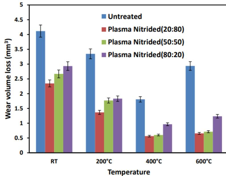
**Figure 10.** The wear volume loss of untreated and plasma-nitrided AISI H13 steel specimens after the wear test.
