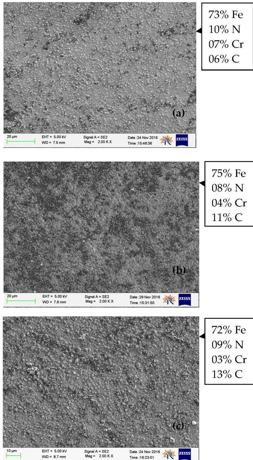
**Figure 4.** Surface-scale morphology and EDS analysis of AISI H13 plasma-nitrided with N<sub>2</sub>:H<sub>2</sub> ratios of (a) 20:80, (b) 50:50 and (c) 80:20.
