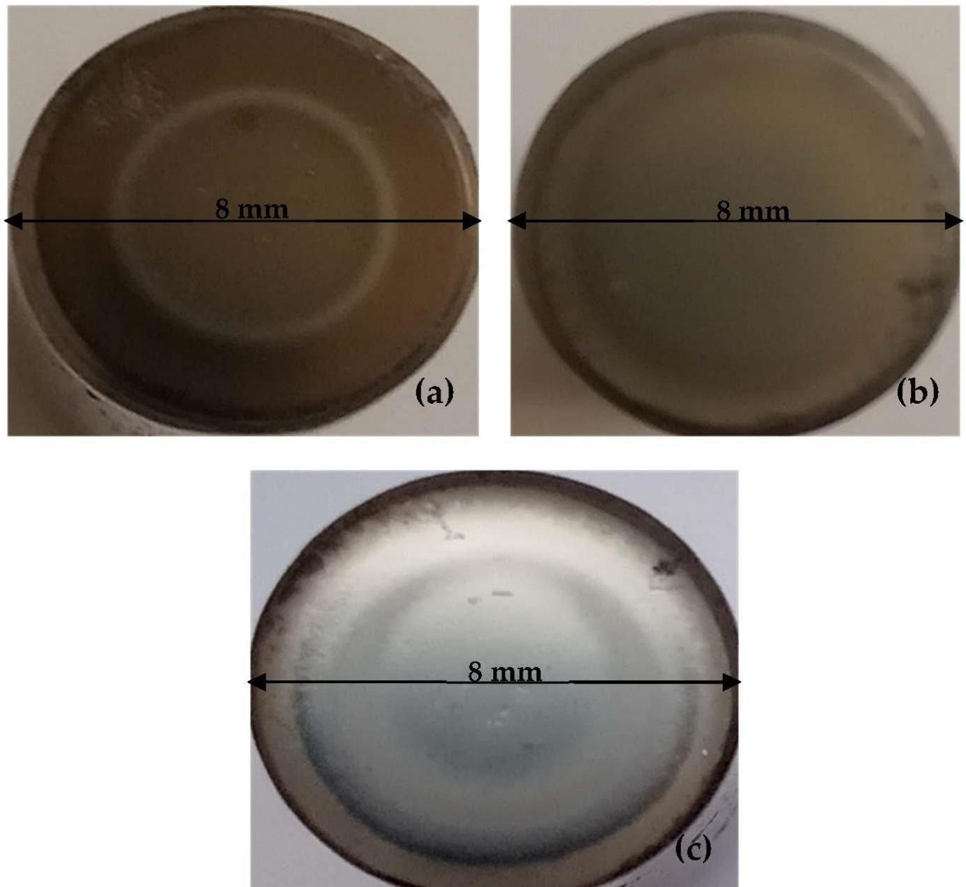
**Figure 3.** Macrographs of AISI H13 plasma-nitrided at 500 °C with  $N_2:H_2$  ratios of (a) 20:80, (b) 50:50, and (c) 80:20 and a 24 h nitriding time.
