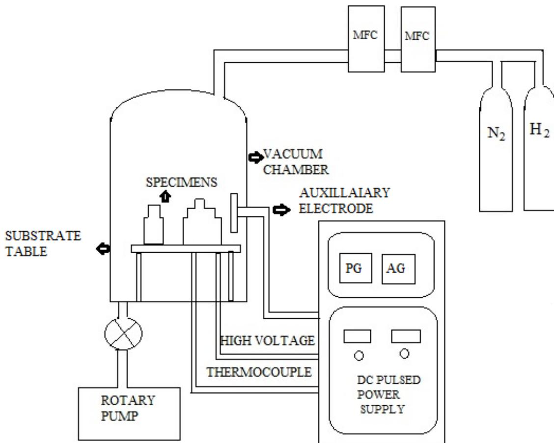
**Figure 1.** Schematic diagram of plasma nitriding set-up. MFC = mass flow controller.
