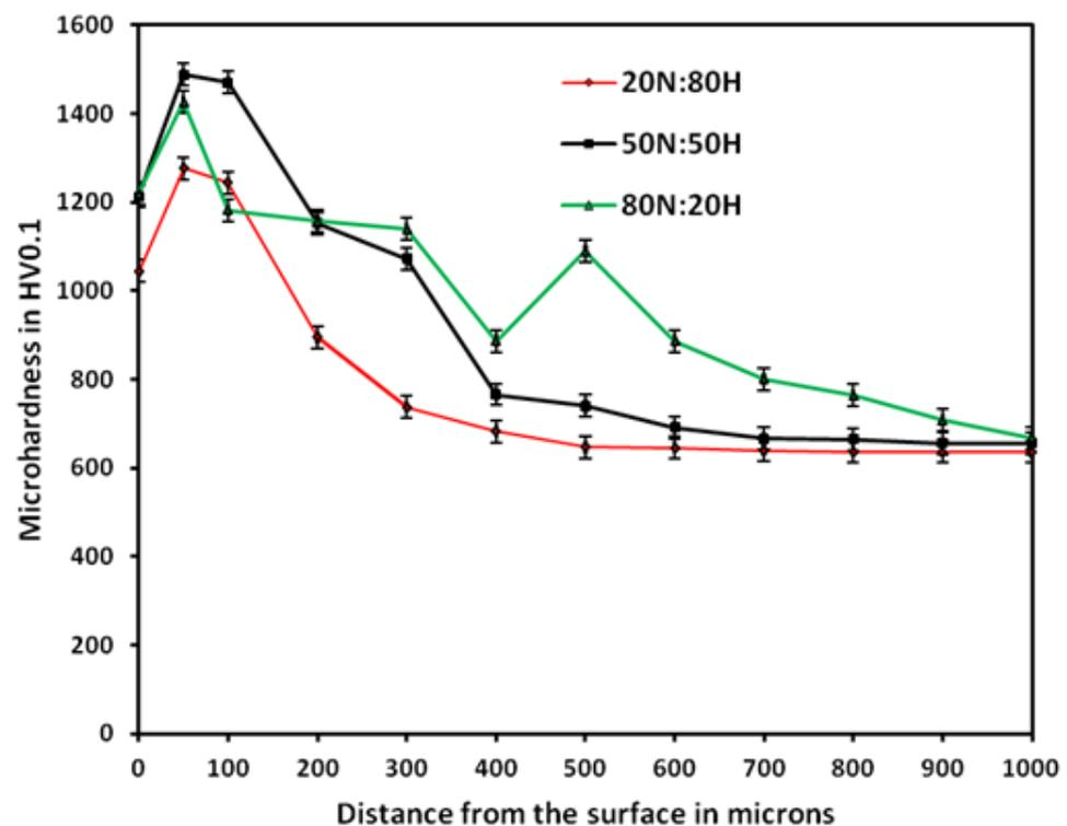
Figure 5. Microhardness depth profile of AISI H13 plasma-nitrided samples.
