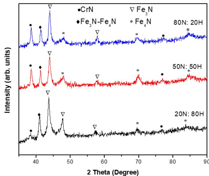
**Figure 7.** X-ray diffraction pattern for the plasma-nitrided AISI H13 steel at 500 °C for 24 h using different gas ratios: blue for 80N<sub>2</sub>:20H<sub>2</sub>; red for 50N<sub>2</sub>:50H<sub>2</sub> and black for 20N<sub>2</sub>:80H<sub>2</sub>.
