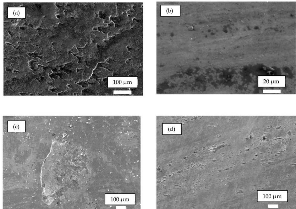
**Figure 11.** The SEM micrographs of worn surfaces of AISI H13 steel specimens after the wear test at RT and under a 50 N load. (a) Heat-treated specimen. (b) PN with 20N<sub>2</sub>:80H<sub>2</sub>. (c) PN with 50N<sub>2</sub>:50H<sub>2</sub>. (d) PN with 80N<sub>2</sub>:20H<sub>2</sub>.
