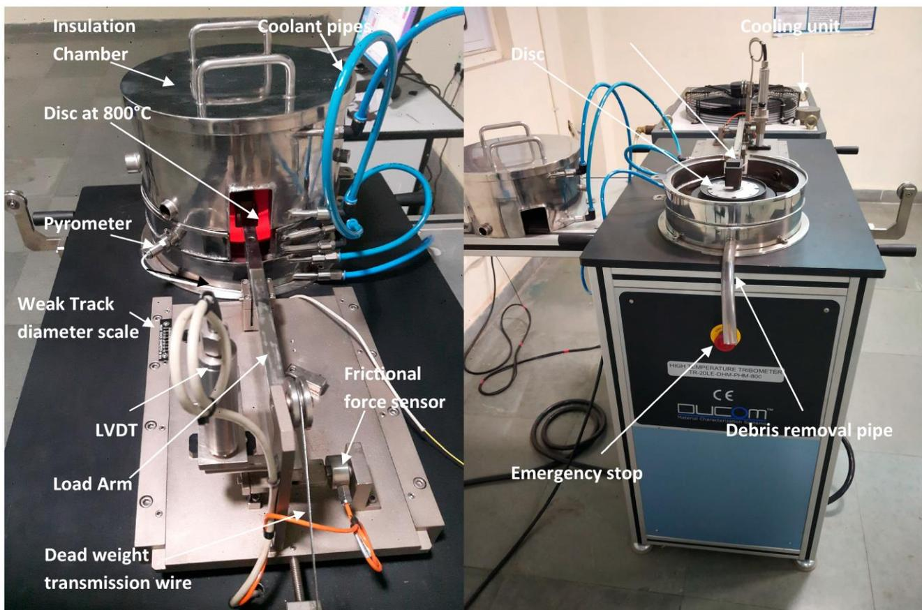
Figure 2. High-temperature pin-on-disc wear and friction tester.
