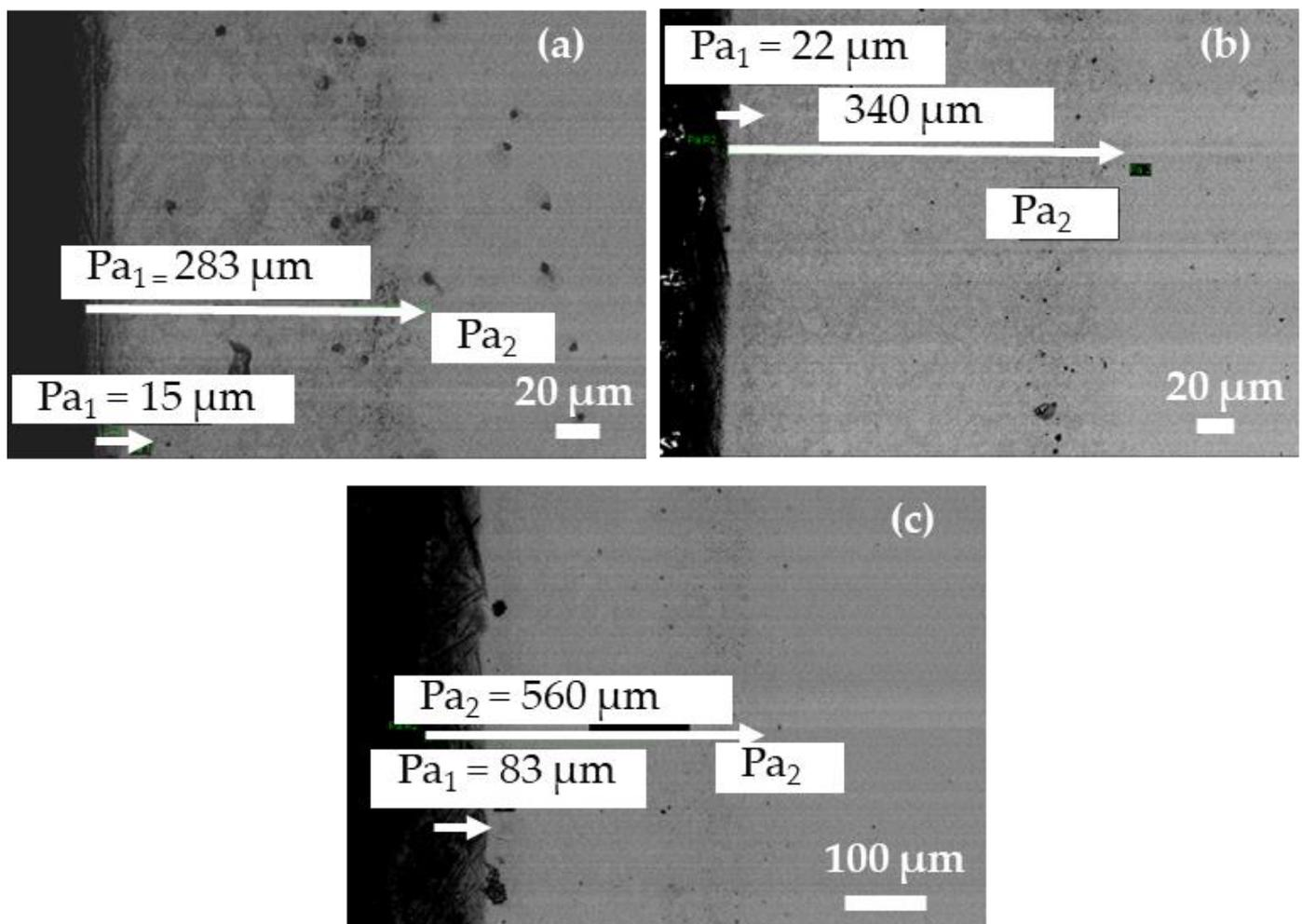
**Figure 6.** Cross-sectional SEM morphology of plasma-nitrided AISI H13 treated at 500 °C for 24 h using (a) 20% nitrogen and 80% hydrogen, (b) 50% nitrogen and 50% hydrogen and (c) 80% nitrogen and 20% hydrogen, showing the case depth thickness.
