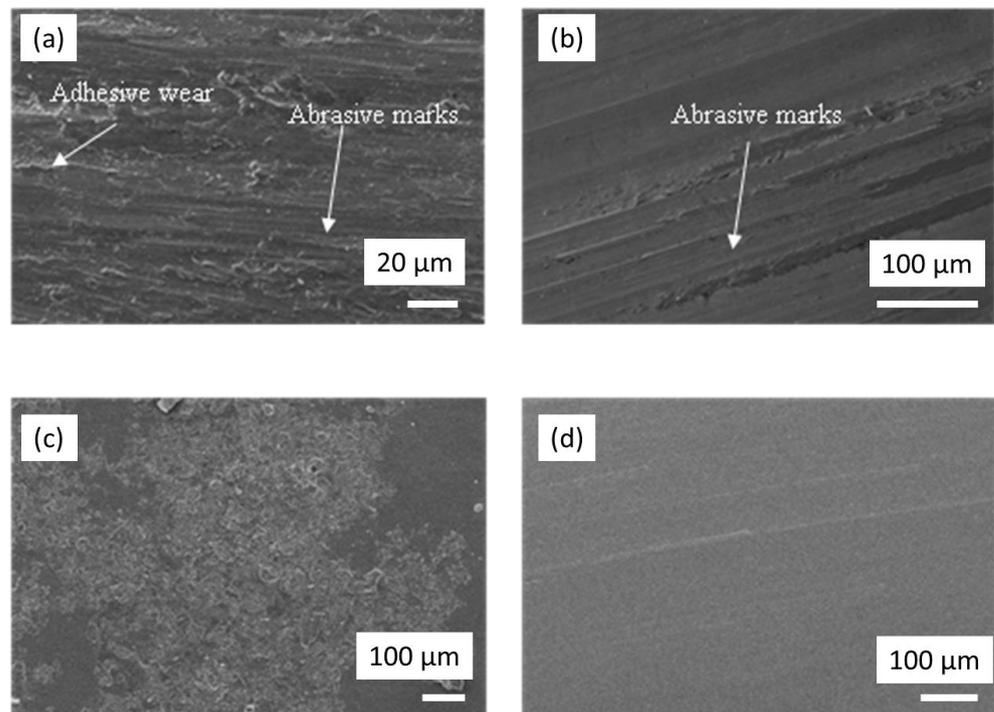
**Figure 13.** The SEM micrographs of worn surfaces of the AISI H13 steel specimens after the wear test at 400 °C and under 50 N loads. (a) Heat-treated specimen. (b) PN with 20N<sub>2</sub>:80H<sub>2</sub>. (c) PN with 50N<sub>2</sub>:50H<sub>2</sub>. (d) PN with 80N<sub>2</sub>:20H<sub>2</sub>.
