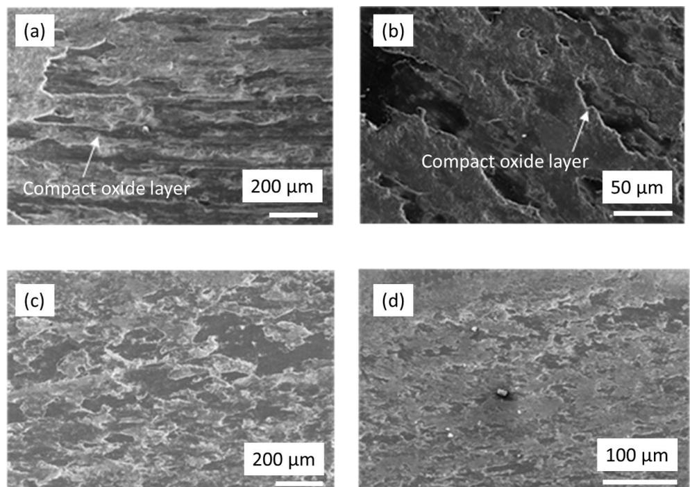
**Figure 14.** The SEM micrographs of worn surfaces of AISI H13 steel specimens after the wear test at 600 °C and under 50 N loads. (a) Heat-treated specimen. (b) PN with 20N<sub>2</sub>:80H<sub>2</sub>. (c) PN with 50N<sub>2</sub>:50H<sub>2</sub>. (d) PN with 80N<sub>2</sub>:20H<sub>2</sub>.
