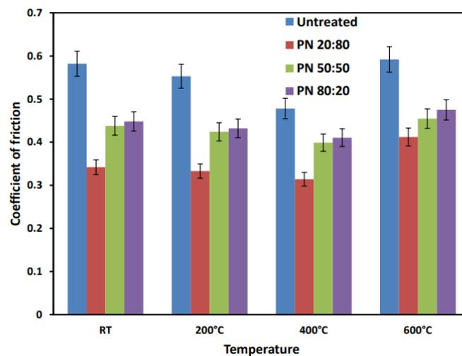
**Figure 9.** The average coefficient of friction of the untreated and plasma-nitrided AISI H13 steel specimens after the wear test.
