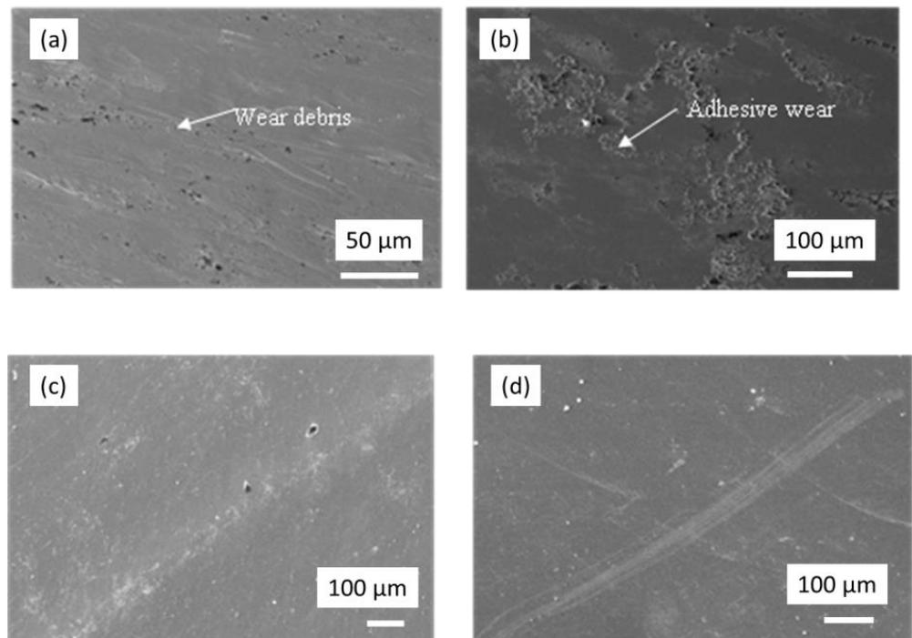
**Figure 12.** The SEM micrographs of worn surfaces of AISI H13 steel specimens after the wear test at 200 °C and under 50 N loads. (a) Heat-treated specimen. (b) PN with 20N<sub>2</sub>:80H<sub>2</sub>. (c) PN with 50N<sub>2</sub>:50H<sub>2</sub>. (d) PN with 80N<sub>2</sub>:20H<sub>2</sub>.
