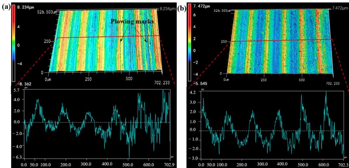
**Figure 8.** Three-dimensional images ( $\times 400$ ) of the surface morphology of (a) CT and (b) UVAT processes under MQL condition.
