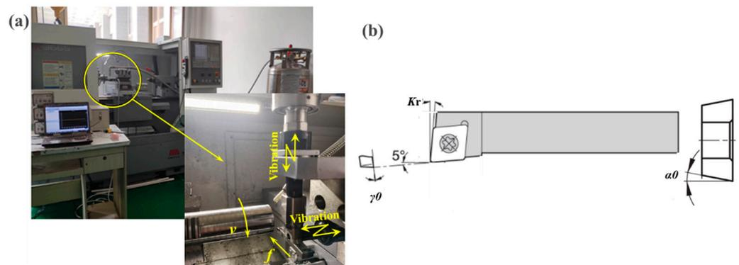
**Figure 2.** (a) Experimental equipment of the UVAT and NMQL method and (b) the cutting tool angles.
