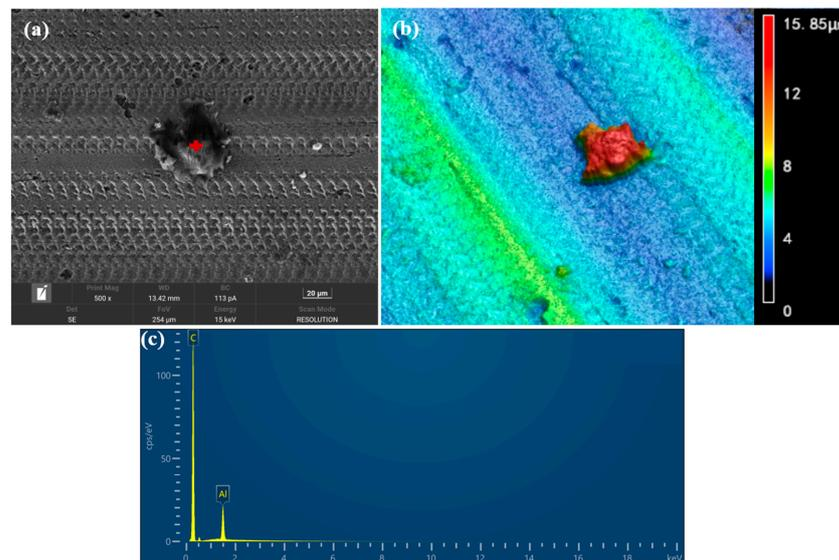
**Figure 4.** (a) SEM and (b) 3D images ( $\times 1000$ ) of the surface morphology of the UVAT and DN-MQL method, and (c) EDS results of the bulge.
