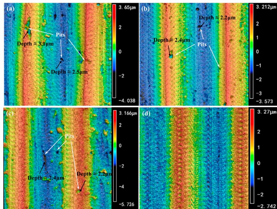
**Figure 9.** Three-dimensional images ( $\times 1000$ ) of the surface morphology of UVAT processes under (a) DN-MQL, (b) GN-MQL, (c) GN+DN-MQL, and (d) MQL conditions.
