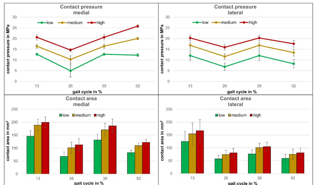
**Figure 4.** Contact pressure and contact area for the low, medium, and high loading condition between the medial, as well as lateral, condyle and the polyethylene insert.
