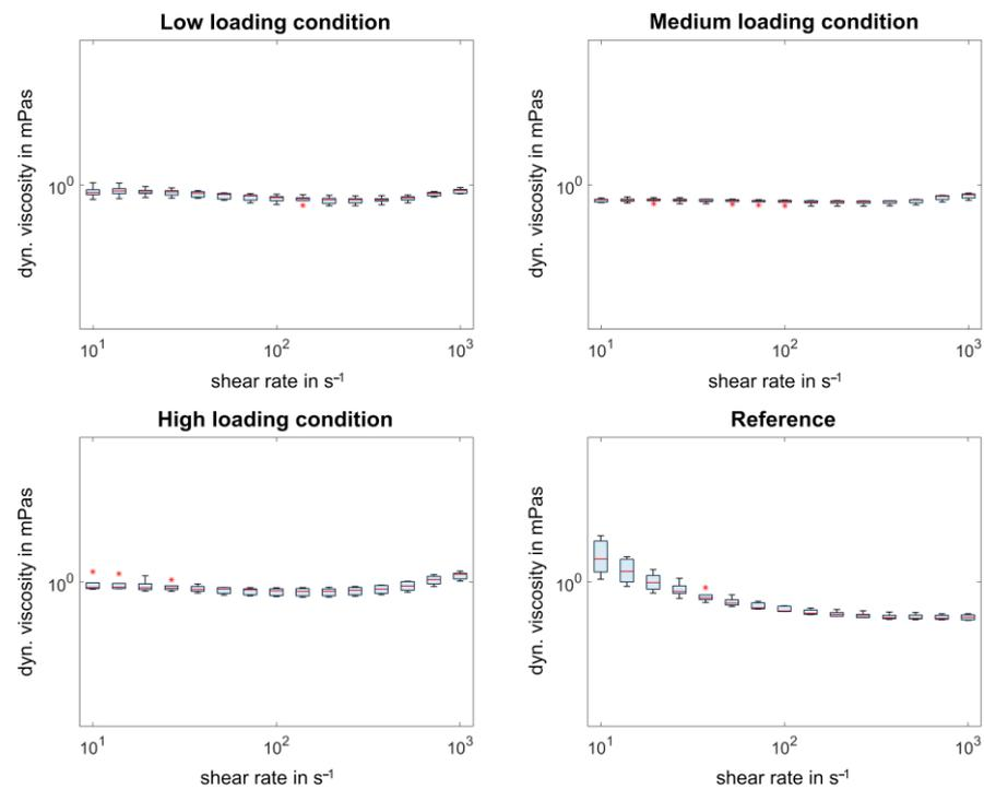
**Figure 6.** Boxplot graphs for the dynamic viscosity as a function of the shear rate for the low, medium, and high loading condition, as well as the reference fluid. Outliers are shown by a red star and they are defined by values that are more than 1.5 times of the interquartile range away from the top or bottom of a box.
