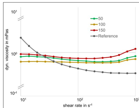
**Figure 5.** Dynamic viscosity as a function of the shear rate for the low, medium, and high loading condition, as well as the reference fluid.
