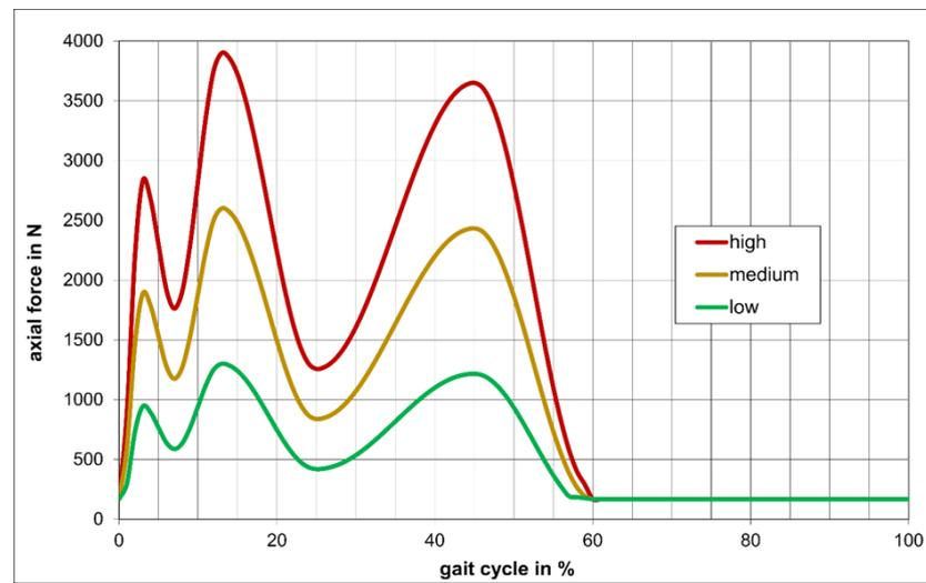
**Figure 1.** Applied load curves for the low, medium, and high loading condition.
