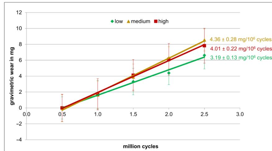
**Figure 3.** Wear rates for the low, medium, and high-load levels.
