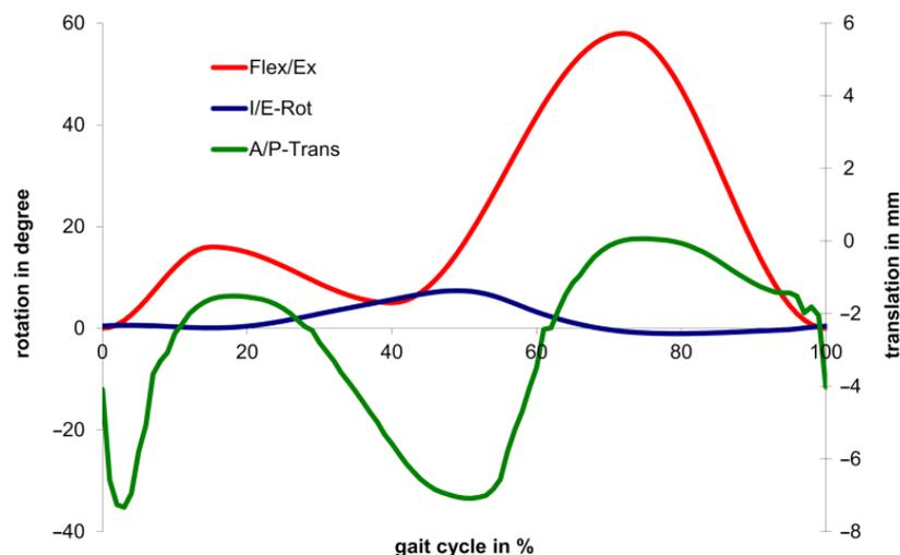
**Figure 2.** Applied kinematics, separated in flexion and extension (Flex/Ex), internal and external rotation (I/E-Rot), as well as translation in the anterior–posterior direction (A/P-Trans).
