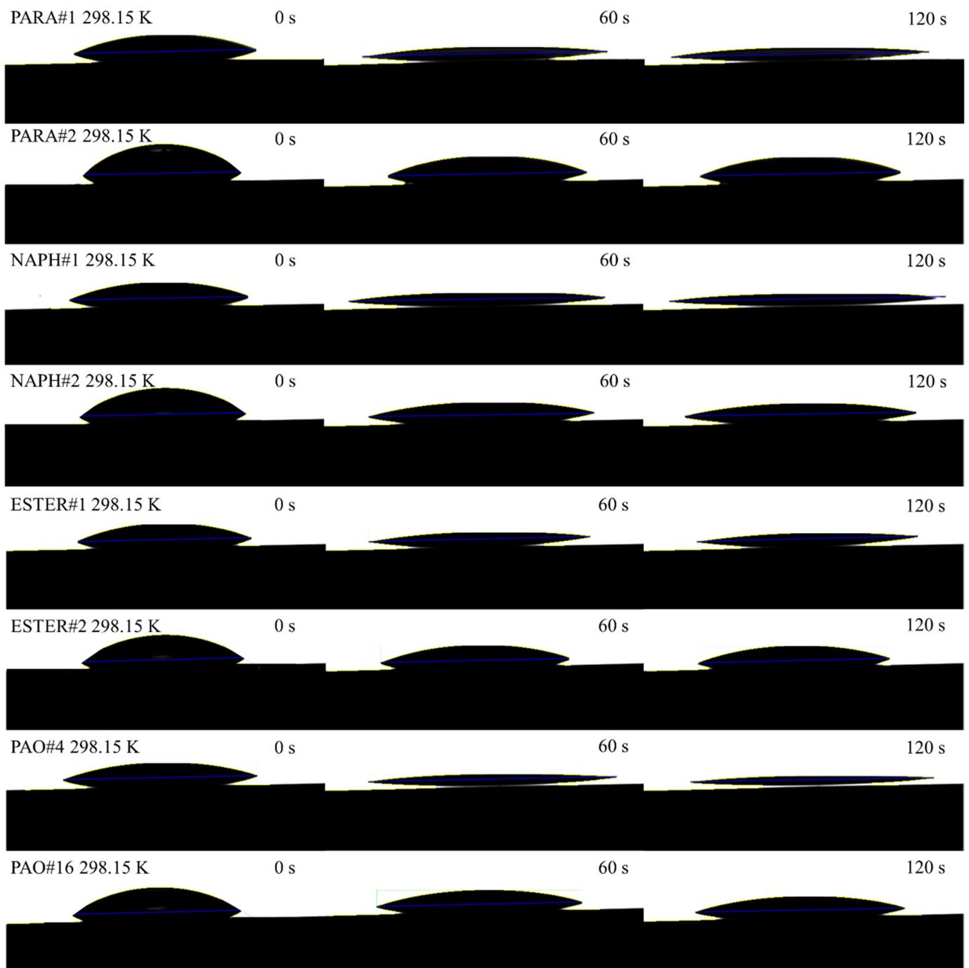
**Figure 7.** Images of the sessile drop evolution for all mineral and synthetic oils at 298.15 K.
