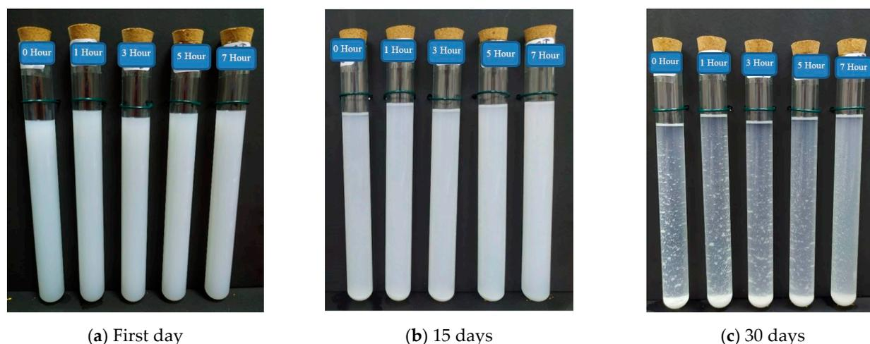
**Figure 3.** Visual observation for ultrasonication bath preparation at different sonication times.
