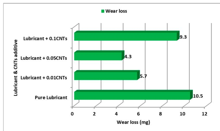
Figure 6. Wear Loss Profiles of Lubricant with CNTs Additives [142].
