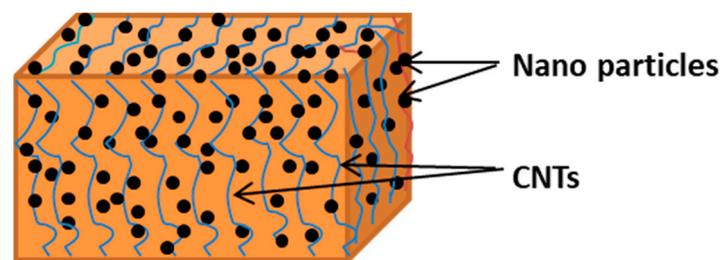
**Figure 2.** Image of CNTs-Reinforced Nanocomposite.
