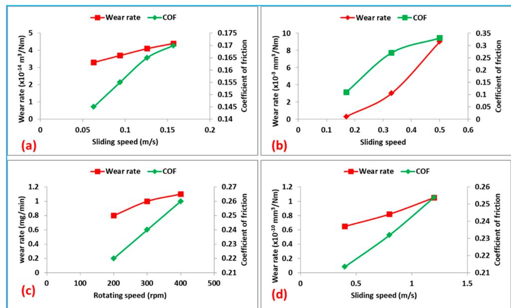
**Figure 3.** Effect of Sliding Speed on the Wear rate and Coefficient of Friction of: (a) Cu-0.5Al<sub>2</sub>O<sub>3</sub>-1.5CNTs, (b) Al<sub>2</sub>O<sub>3</sub>-3TiO<sub>2</sub>-6CNTs, (c) Glass Fiber-Reinforced Plastic-1CNTs and (d) Polyamide-30Carbon fiber-0.5CNTs Composites [74,82,91,92].
