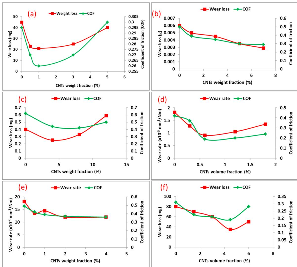
**Figure 5.** Effect of Volume Fractions of CNTs on Wear Loss and COF of (a) Polypropylene-CNTs, (b) Polypropylene-CNTs, (c) Alumina-CNTs, (d) Cu-CNTs, (e) Mg-CNTs and (f) Al-CNTs Composites, Adapted from [35,101,104–107].
