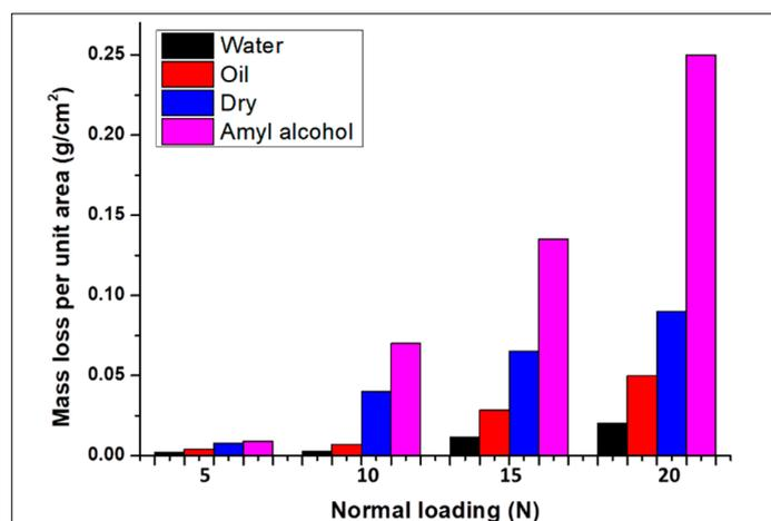
**Figure 4.** Comparison of Wear Loss of Ceramics–Carbide Composites on Different Lubricants, Adapted from [99].
