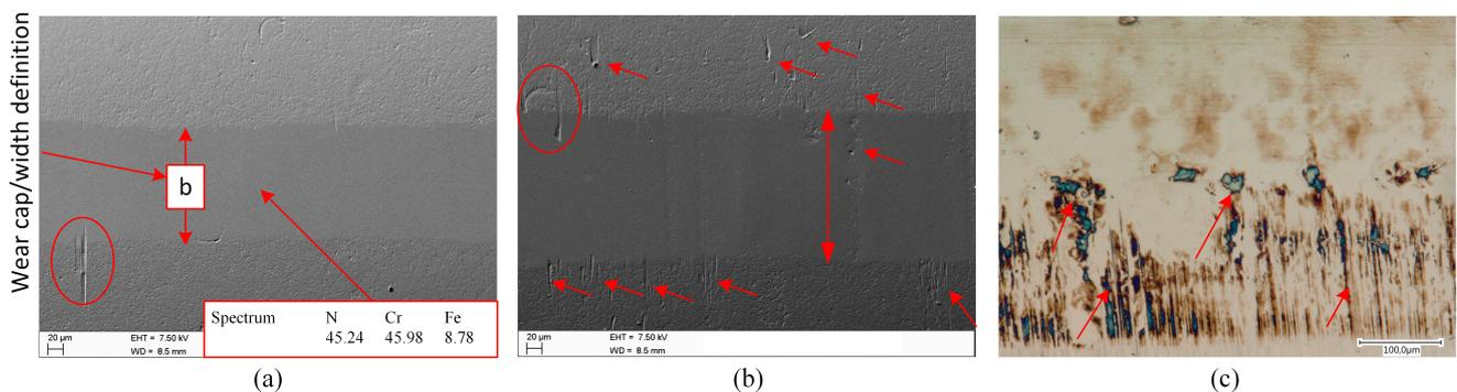
**Figure 8.** Surface analysis of selected test parts with EO1/Cr-N-Fe test combination: (a) Pin surface from test with TC 1 test programme (measured with 7.5 kV and values given in at.%); (b) Pin surface from test with TC 2 test programme; (c) Steel counterpart surface from test with TC 2 test programme. In the illustrations, the arrows and the red circles mark abrasive grooves (a,b) as well as regions of tribofilm formation for (c). The b label shows the wear cap.
