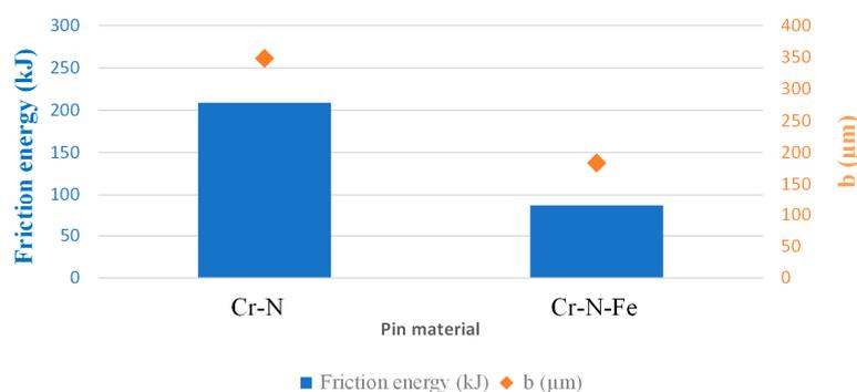
**Figure 11.** Quantitative results regarding friction energy ( $E_f$ ) and wear (wear width  $b$ ) from tests with EO2 lubricant.
