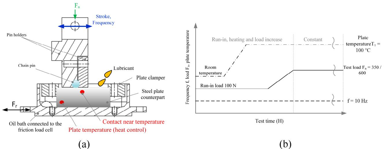
**Figure 1.** Test method details: (a) Schematic of the test set up; (b) Test programme (Adapted from [1]).
