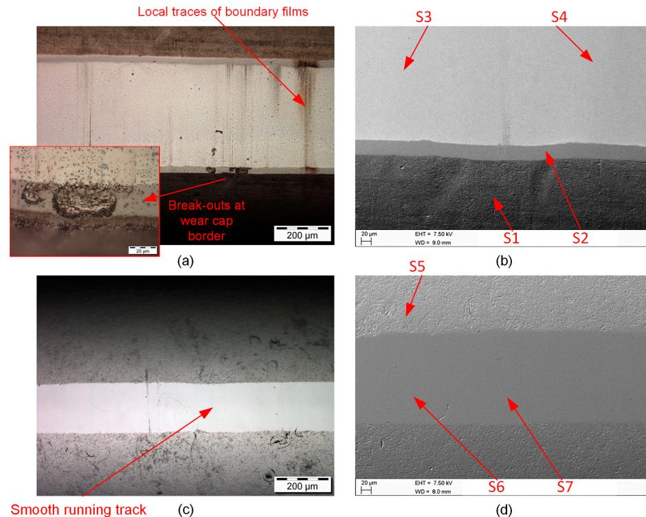
**Figure 12.** Pin surfaces from tests with EO2 lubricant obtained with TC 4 test programme: (a) LIM image of Cr-N; (b) SEM image of Cr-N; (c) LIM image of Cr-N-Fe; (d) SEM image of Cr-N-Fe.
