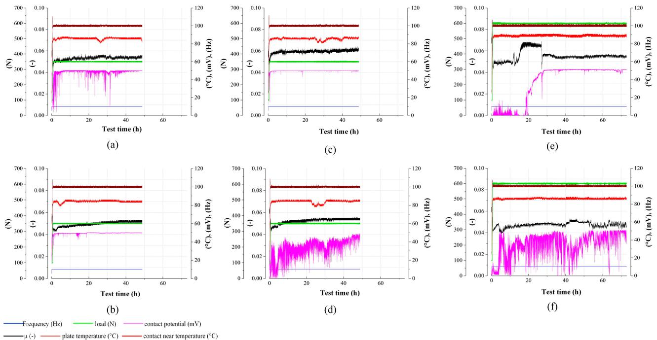
**Figure 14.** Tests with artificial lubricants without soot: (a) Cr-N material and AO1 for TC 4 programme; (b) Cr-N-Fe material and AO1 for TC 4 programme; (c) Cr-N material and AO3 for TC 4 programme; (d) Cr-N-Fe material and AO3 for TC 4 programme; (e) Cr-N material and AO3 for TC 5 programme; (f) Cr-N-Fe material and AO3 for TC 5 programme.
