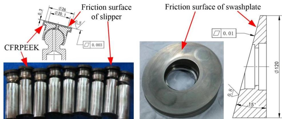
**Figure 2.** Slipper and swashplate parts of WLPP.
