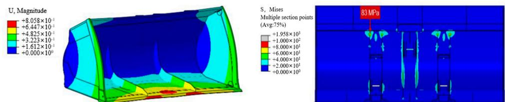
Figure 8. Stress (left) and pressure nephogram (right) under horizontal positive load conditions.
