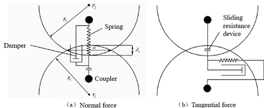
Figure 7. Hertz–Mindlin contact model.
