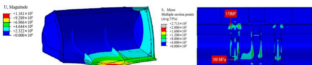
Figure 10. Stress (left) and pressure nephogram (right) under vertical off-load conditions.
