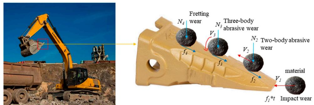
Figure 2. Tooth wear diagram of bucket.
