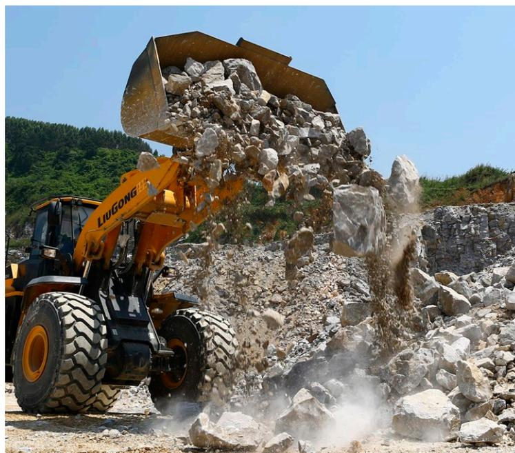
**Figure 5.** Working conditions with abrasive wear governed.
