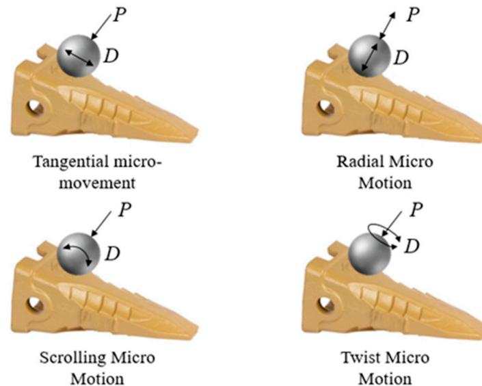
**Figure 6.** The basic form of micro-movement of the material on the bucket teeth [26].
