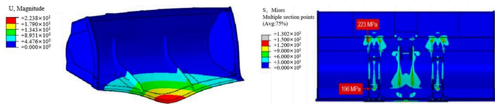
**Figure 11.** Stress (left) and pressure nephogram (right) under horizontal and vertical positive load conditions.
