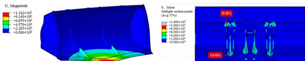
Figure 9. Stress (left) and pressure nephogram (right) under vertical positive load conditions.
