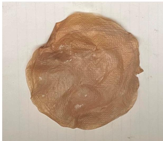
**Figure 9.** The microcellular foamed bacterial cellulose.
