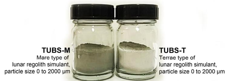
**Figure 1.** TUBS-M and TUBS-T lunar regolith simulants.
