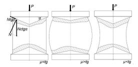
Figure 2. Upsetting process of the conical sample.
