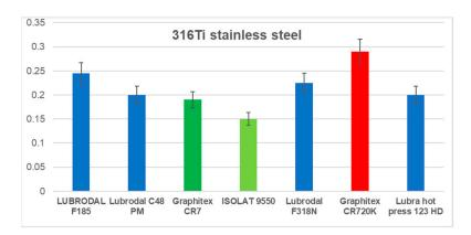
Figure 10. Results of the friction coefficient determination from a ring test for stainless steel.
