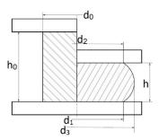
Figure 3. Process of upsetting a cylindrical sample.
