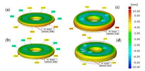
**Figure 12.** Three-dimensional scanning results for (a) a carbon steel sample, for which Lubrodal F318N was used (u = 0.24), (b) a sample with lubrication by means of Lubra hot press 123HD (u = 0.33), (c) a stainless steel sample for which Graphitex CR 7 was applied (u = 0.19) and (d) a sample with lubrication by means of Graphitex CR720K (u = 0.29).
