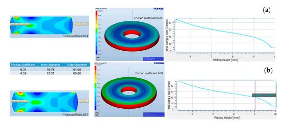
**Figure 13.** Simulation results with the distributions of deformations, unit pressures and forces during upsetting for carbon steel for the extreme friction coefficient values and the internal and external diameter dimensions for (a) u = 0.24 and (b) u = 0.33.
