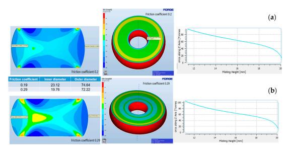
**Figure 14.** Simulation results with the distributions of deformations, unit pressures and forces during upsetting for stainless steel for the extreme friction coefficient values and the internal and external diameter dimensions for (**a**) u = 0.2 and (**b**) u = 0.29.
