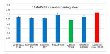
Figure 11. Results of the friction coefficient determination from a ring test for carbon steel.
