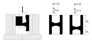
Figure 5. Double Cup Extrusion -process of forward-backward extrusion.
