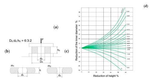
**Figure 6.** View of (a) a diagram of the ring upsetting process and the dimensions of samples after upsetting for different friction coefficient values, (b) poor lubrication  $d_1 > d_0$ , (c) good lubrication  $8d_2 < d_0$ ,  $m_2 > m_1$ , and (d) nomogram for friction coefficient readings.
