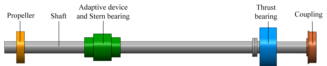
Figure 3. Configuration of propulsion system with adaptive vibration-damping device.
