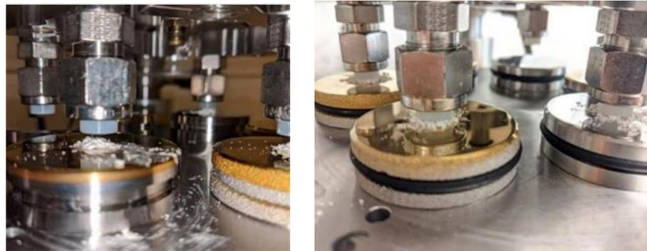
**Figure 5.** 14 mg of PMMA particles were loaded below each UHMWPE pin. The pins were lowered and brought into contact with the PMMA particles. Running-in included an initial 1000-cycle dry run, followed by the repositioning of expelled particles and an additional 1000 cycles before the lubricant (described under Section 2.4.1) was introduced.
