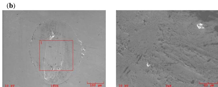
**Figure 10.** SEM micrographs of the wear scars on AISI 52100 steel flat disks ( $R_a \approx 0.02 \mu\text{m}$ ) after a ball-on-flat reciprocating test using the following lubricants: (a) PAO; (b) PAO + 5% [THTDP][NTf2].
