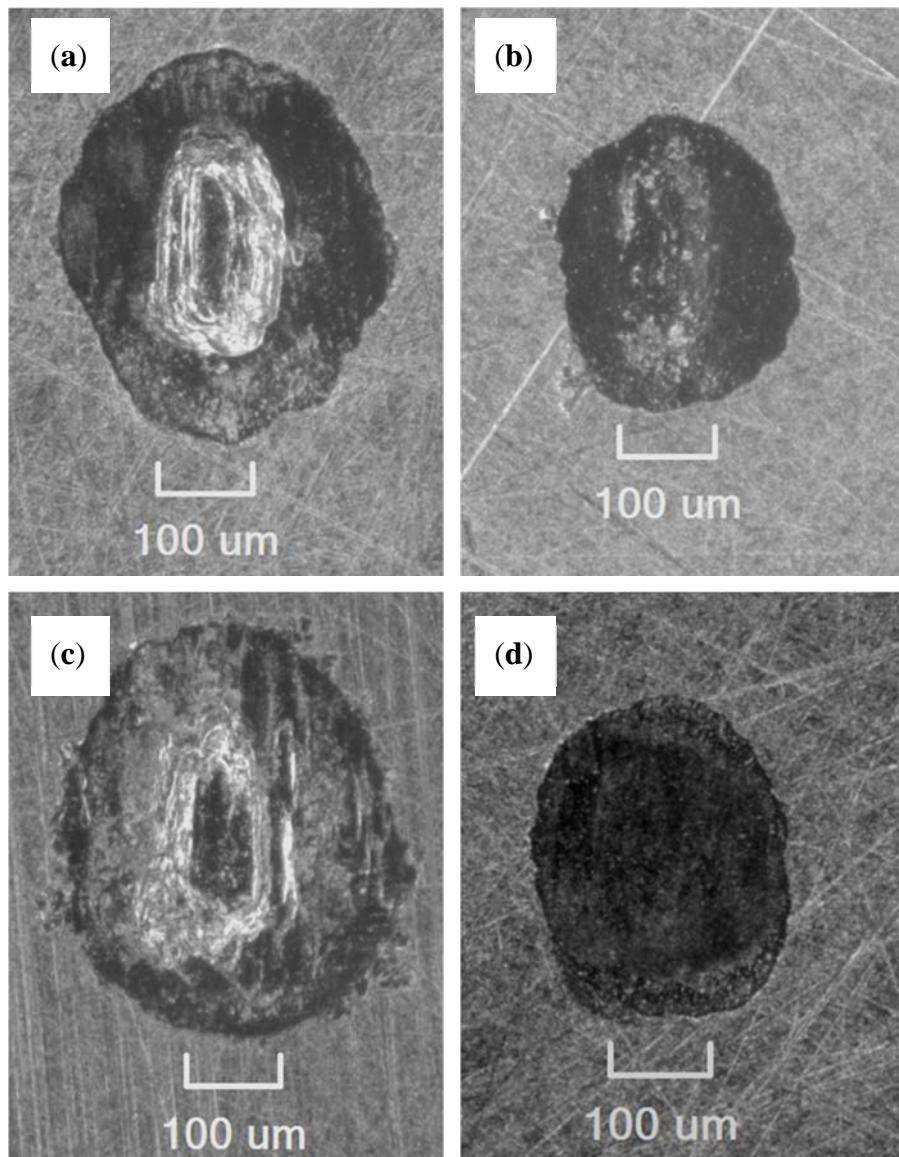
**Figure 4.** Wear scars on AISI 52100 steel flat disks ( $R_a \approx 0.1 \mu\text{m}$ ) after a ball-on-flat reciprocating test using the following lubricants: (a) MG; (b) MG + 5% [THTDP][NTf2]; (c) PAO; and (d) PAO + 5% [THTDP][NTf2].
