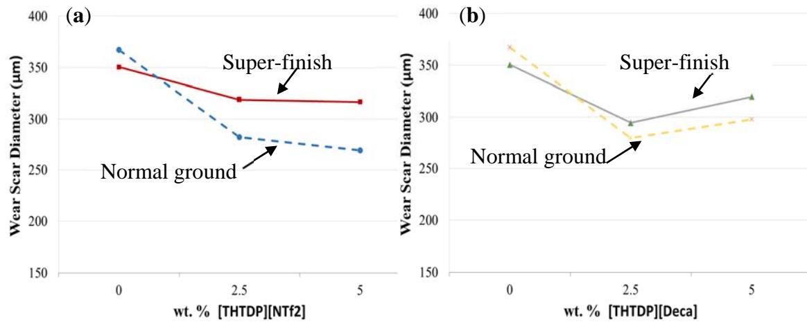
**Figure 7.** Wear scar diameters on AISI 52100 steel flat disks for both surface finishes after a ball-on-flat reciprocating test using PAO as base lubricant and (a) [THTDP][NTf2], and (b) [THTDP][Deca] as an additive.
