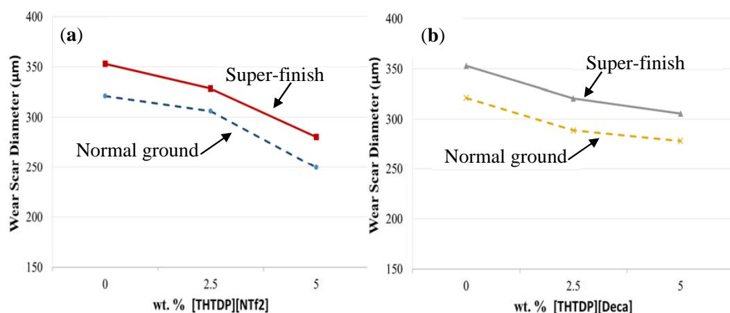
**Figure 6.** Wear scar diameters on AISI 52100 steel flat disks for both surface finishes after a ball-on-flat reciprocating test using MG as base lubricant and (a) [THTDP][NTf<sub>2</sub>], and (b) [THTDP][Deca] as an additive.
