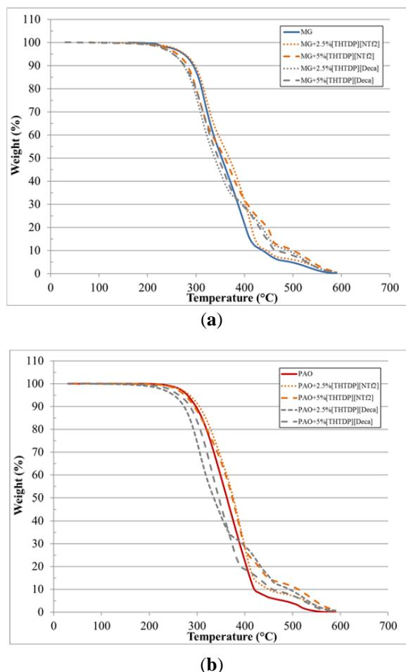
**Figure 2.** Weight loss vs. temperature thermogravimetric analysis (TGA) curves for the lubricants: (a) Mobilgear SHC XMP 320 (MG) and MG mixtures with ILs; (b) Synton PAO-40 (PAO) and PAO mixtures with ILs.
