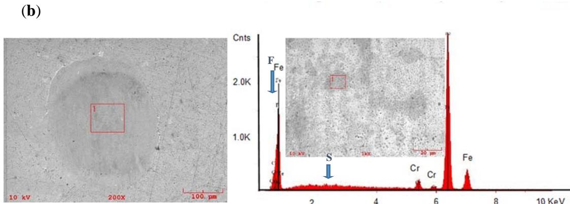
**Figure 5.** SEM micrographs and energy-dispersive X-ray spectroscopy (EDS) analysis of the wear scars on AISI 52100 steel flat disks ( $R_a \approx 0.1 \mu\text{m}$ ) after a ball-on-flat reciprocating test using the following lubricants: (a) PAO; (b) PAO + 5% [THTDP][NTf<sub>2</sub>].
