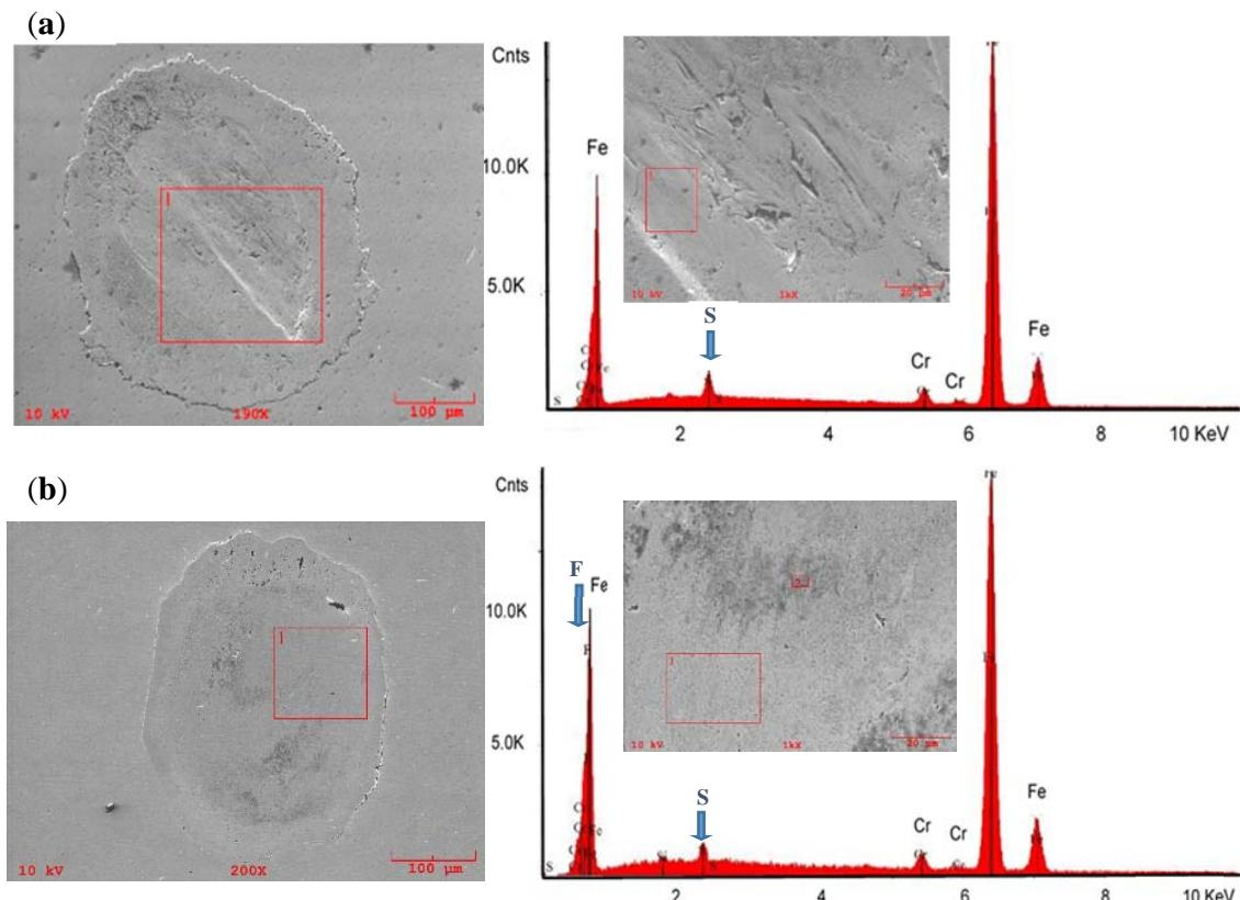
**Figure 9.** SEM micrographs and EDS analysis of the wear scars on AISI 52100 steel flat disks ( $R_a \approx 0.02 \mu\text{m}$ ) after a ball-on-flat reciprocating test using the following lubricants: (a) MG; (b) MG + 5% [THTDP][NTf2].
