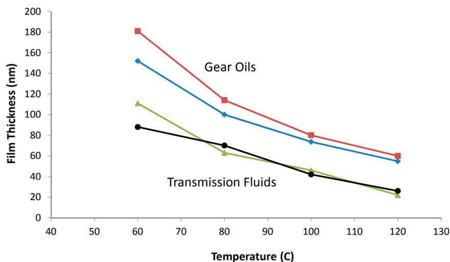
Figure 4. Effect of temperature on film thickness for two different gear oils and two different transmission fluids.
