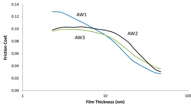
**Figure 6.** Friction versus film thickness for lubricants with different anti-wear (AW) additives.
