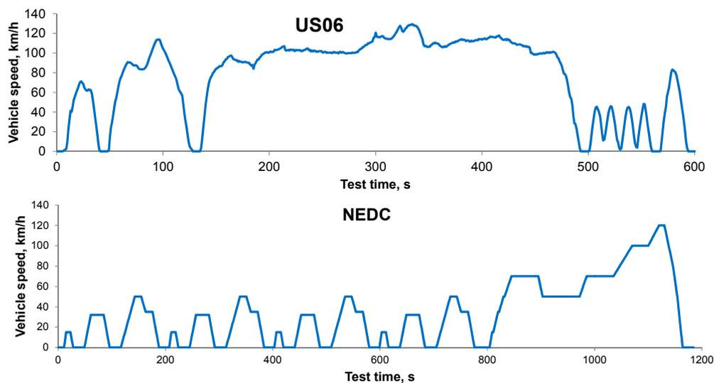
**Figure 2.** Driving cycles used to measure vehicle fuel economy. NEDC = New European Driving Cycle.
