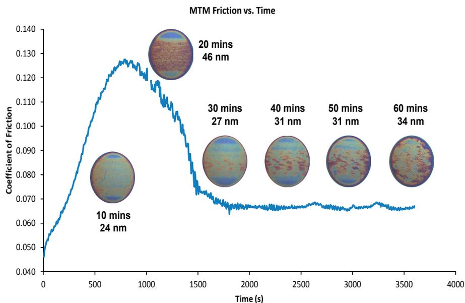
**Figure 8.** Changes in Mini-Traction Machine (MTM) friction as tribofilms form.
