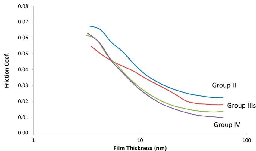
Figure 5. Friction versus film thickness for four different base oils.
