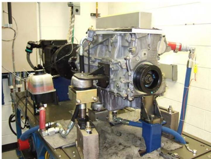
**Figure 6.** Experimental set-up for cranktrain friction measurements.
