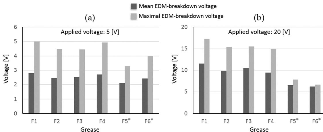
**Figure 10.** The maximum and mean EDM breakdown voltage occurring at an applied test voltage amplitude for all investigated lubricants; (a) results at an applied test voltage of 5 V; (b) results at an applied test voltage of 20 V (\* conductive greases).
