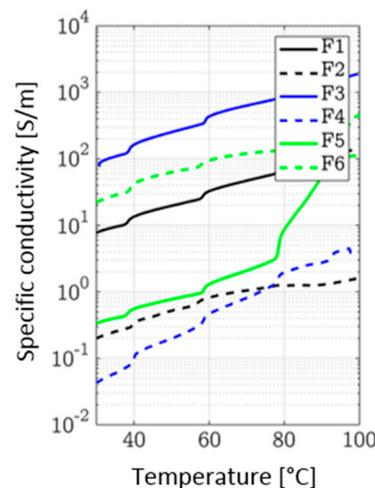
**Figure 6.** Measured specific conductivity of the test greases at switching frequency of 20 Hz, temperature from 30 to 100 °C and at a pressure of 1 bar in a cylinder capacitor.
