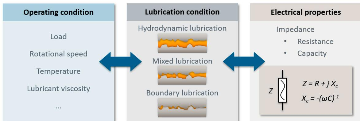
**Figure 1.** Relationship between the operating condition, the corresponding lubrication condition, and its electrical properties in rolling bearing.
