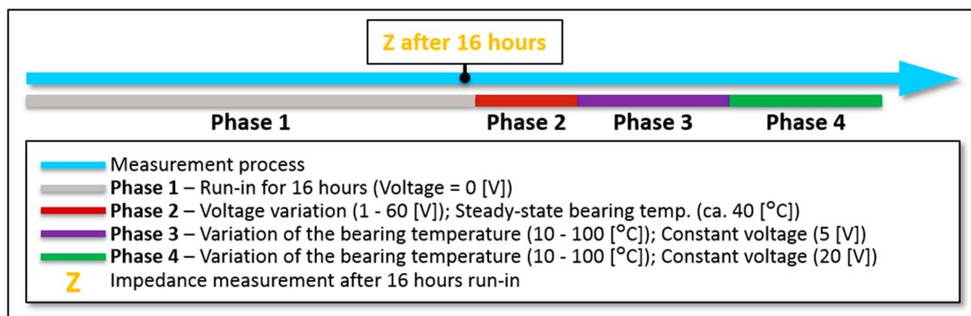
**Figure 5.** The measurement process for the investigated lubricants.
