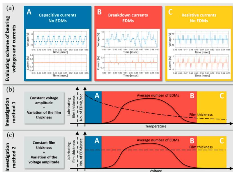
**Figure 3.** (a) Evaluating scheme of the bearing voltages and currents; (b) investigation method 1 of the bearing currents; (c) investigation method 2 of the bearing currents.
