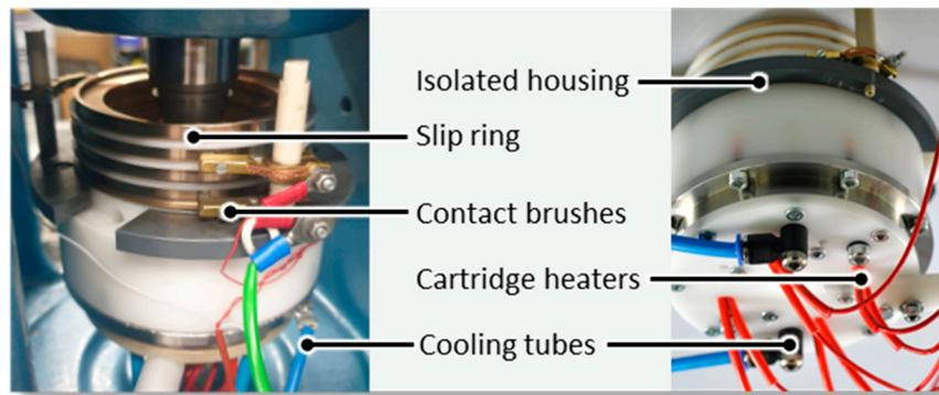
**Figure 4.** The assembly of the GESA test cell.
