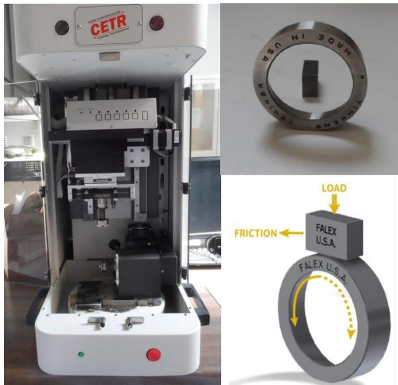
**Figure 1.** Tribometer and specimens used for the wear tests.
