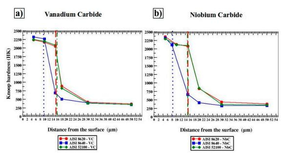
**Figure 6.** Microhardness profiles of (**a**) vanadium carbide (VC) and (**b**) niobium carbide (NbC) layers produced for 4 h. The vertical lines represent the approximate thickness of the coatings on AISI 8620 (dash line), 8640 (dot line), and 52100 (dash-dot line).
