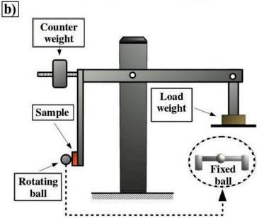
**Figure 1.** Schematic representation of the (a) profile hardness in the cross section of the sample and (b) microadhesive wear of the calotest type.
