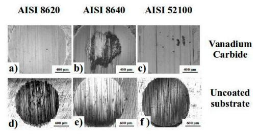
**Figure 8.** Optical micrographs of wear regions inside the caps produced on vanadium carbide (VC) (**a–c**) layers and uncoated substrates (**d**) AISI 8620, (**e**) 8640, and (**f**) 52100 treated for 4 h.
