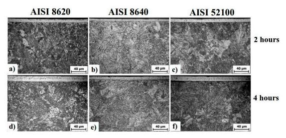
**Figure 3.** Optical micrographs of niobium carbide (NbC) layers produced on AISI 8620 (**a**,**d**), 8640 (**b**,**e**) and 52100 (**c**,**f**) steels at 1000 °C for 2 h (**a**-**c**) and 4 h (**d**-**f**).
