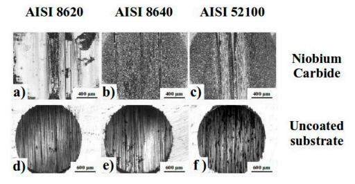
**Figure 9.** Optical micrographs of wear regions inside the caps produced on niobium carbide (NbC) (**a–c**) layers and uncoated substrates (**d**) AISI 8620, (**e**) 8640, and (**f**) 52100 treated for 4 h.
