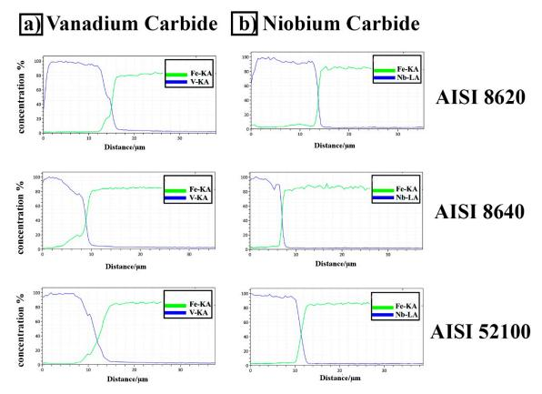
**Figure 5.** EDS depth profiles of (**a**) vanadium carbide and (**b**) niobium carbide layers produced on AISI 8620, 8640, and 52100 steels for 4 h.
