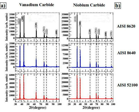
**Figure 4.** X-ray diffraction of vanadium carbide (VC) and niobium carbide (NbC) layers formed on AISI 8620, 8640, and 52100 steels treated for 4 h. Dashed lines represent the position of VC and NbC references, respectively.
