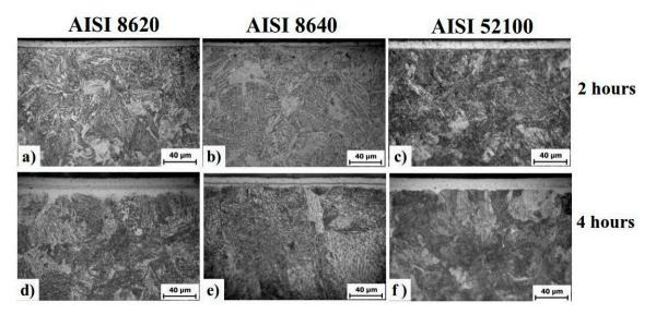
**Figure 2.** Optical micrographs of vanadium carbide (VC) layers produced on AISI 8620 (**a**,**d**), 8640 (**b**,**e**) and 52100 (**c**,**f**) steels at 1000 °C for 2 h (**a**-**c**) and 4 h (**d**-**f**).
