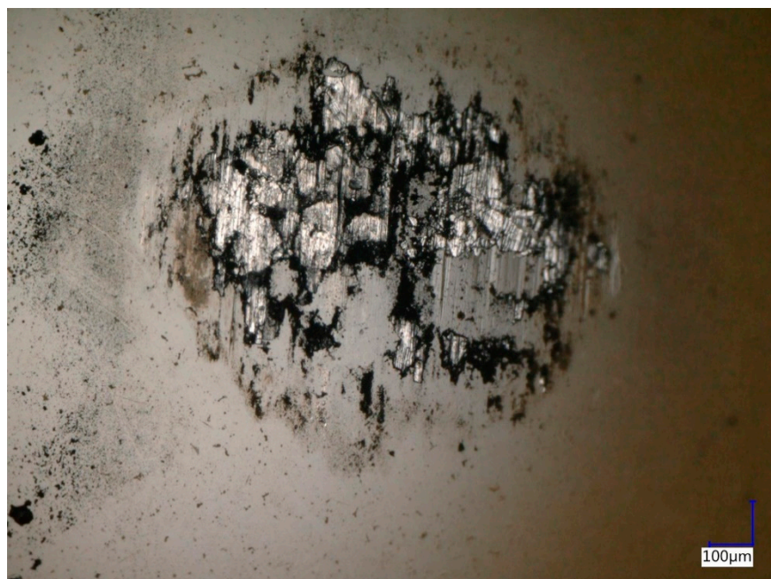
Figure 23. Wear marks on the surface of \text{ZrO}_2 ball after sliding against the uncoated CoCrMo disc, F_n : 100 N, f : 1 Hz, dry (2D image, digital microscopy).
