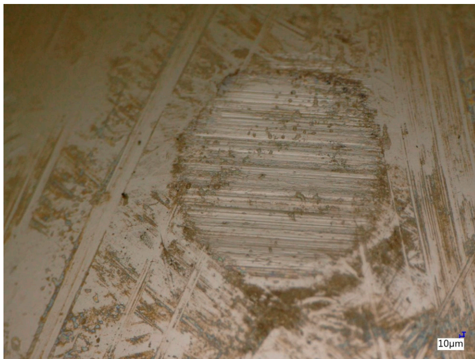
Figure 25. Wear marks on the surface of \text{ZrO}_2 ball after sliding against the a-C:H-coated CoCrMo disc, F_n : 100 N, f : 1 Hz, dry (2D image, digital microscopy).
