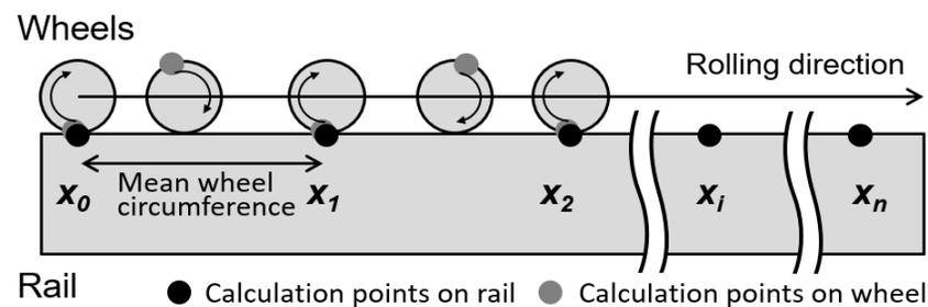
Figure 3. Discretization of wheels and rail.
