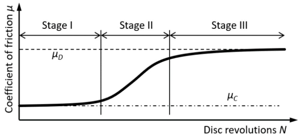
**Figure 5.** Schematic evolution of the coefficient of friction  $\mu$  with the number of disc revolutions  $N$  in a twin disc experiment from an initially low coefficient of friction  $\mu_C$  after the application of product to a high coefficient of friction  $\mu_D$  typical for dry and clean contact conditions without product.
