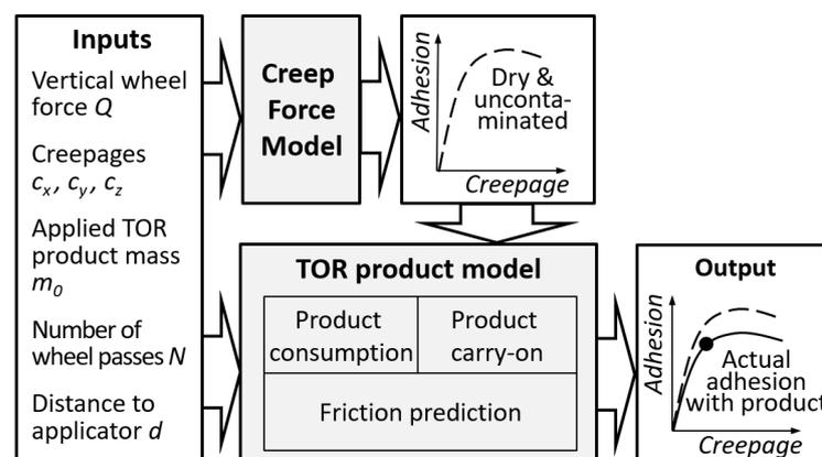
Figure 2. Modelling approach, input data, and output data.
