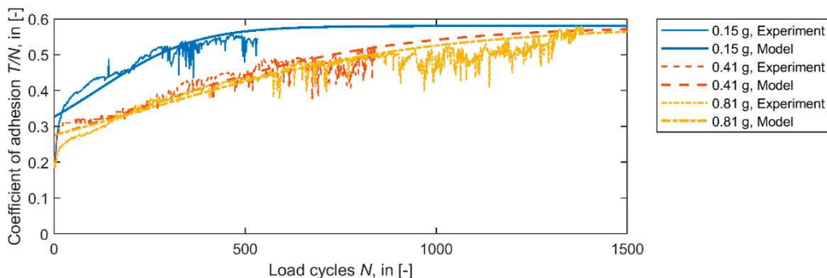
**Figure 11.** Check of the model parameterization for different product amounts; full-scale wheel–rail test rig experiment at 80 kN wheel force and 5% longitudinal creepage; thin lines indicate the experimental data and thick lines indicate the model results.
