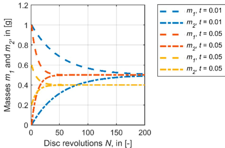
**Figure 8.** Change of product masses  $m_1$  and  $m_2$  with the number of disc revolutions  $N$  due to the transfer of product between the surfaces in a twin disc setup. Three examples without product consumption for different transfer function values  $t$  and initial product masses are presented.
