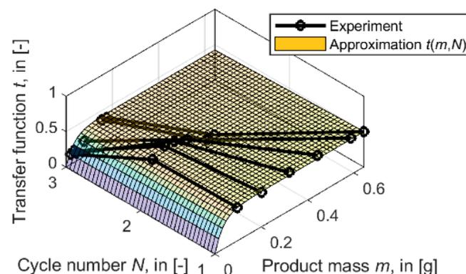
**Figure 12.** Parameterization of the transfer function  $t$  according to Equation (6): pick-up experiments at the full-scale wheel–rail test rig at 80 kN wheel load and 5% longitudinal creepage.
