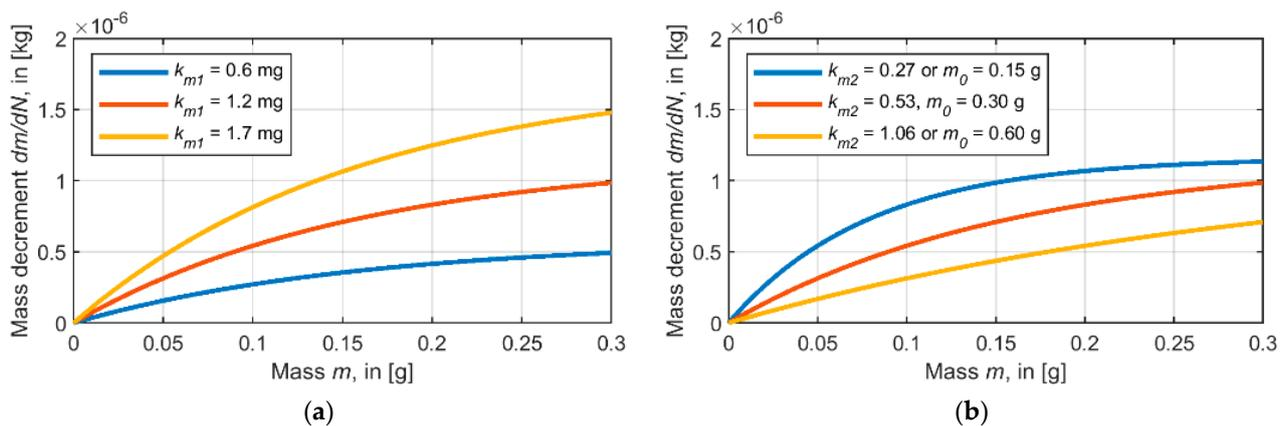
**Figure 4.** Change of product mass decrement  $dm/dN$  according to Equation (1) with  $k_0 = 0$ ,  $f_p = f_c = 1$ : (a)  $k_{m2} = 0.53$ , variation of  $k_{m1}$ , and (b)  $k_{m1} = 1.2$  mg, variation of  $k_{m2}$  or applied product mass  $m_0$ .
