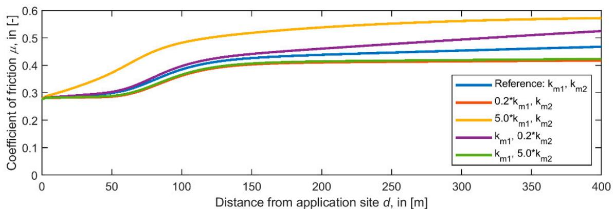
**Figure 16.** Coefficient of friction  $\mu$  as a function of the distance from the application site  $d$ . Variation of parameters  $k_{m1}$  and  $k_{m2}$  that describe the consumption behaviour according to Equation (1).
