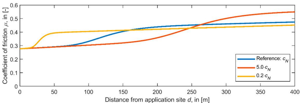
**Figure 15.** Coefficient of friction  $\mu$  as a function of the distance from the application site  $d$ . Variation of parameter  $c_N$  of the transfer function (see Equation (6)).
