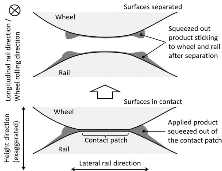
**Figure 9.** Cross-sectional view of the rail and wheel. Bottom: when the wheel and rail are in contact, some product is squeezed out of the contact patch laterally. Top: when the wheel and rail separate, product is carried on near the contact patch edges on the wheel surface, which is partially re-transferred to the rail if contact width and position do not change along the track.
