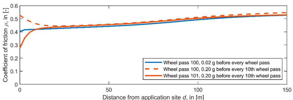
**Figure 17.** Comparison of two product application scenarios: blue solid, wheel pass 100, 0.02 g of product application before every wheel pass.; red dashed, wheel pass 100 (before reapplication), 0.20 g of product application before every 10th wheel pass.; and red solid, wheel pass 101 (after reapplication), 0.20 g of product application before every 10th wheel pass.
