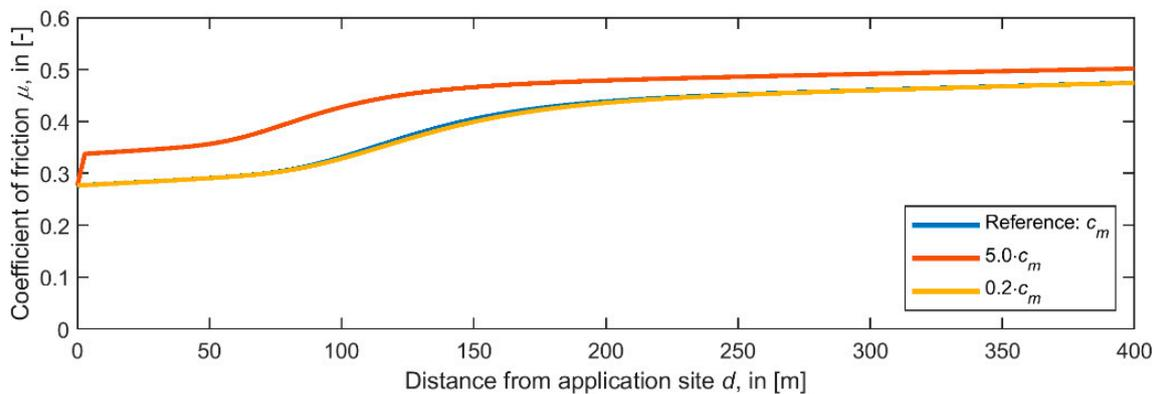
**Figure 14.** Coefficient of friction  $\mu$  as a function of the distance from the application site  $d$ . Variation of parameter  $c_m$  of the transfer function (see Equation (6)).
