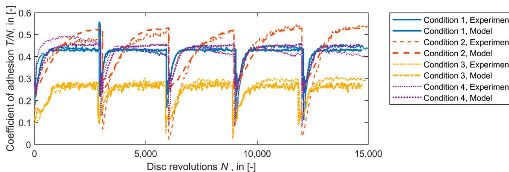
**Figure 10.** Check of the model parameterization, twin disc rig, conditions according to Table 1, model parameters according to Table 2; thin lines indicate the experimental data and thick lines indicate the model results.
