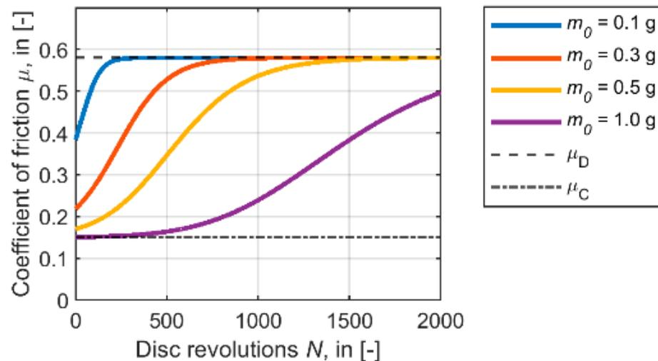
**Figure 7.** Change of coefficient of friction  $\mu$  with the number of disc revolutions  $N$  for different applied product masses  $m_0$  according to Equations (1) and (4) with parameters according to Table 2 in Section 3. Limiting values for dry and clean condition  $\mu_D$  and fully conditioned surface condition  $\mu_C$  are plotted as thin lines.
