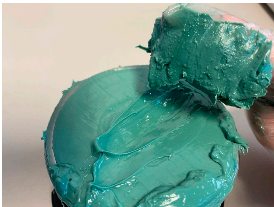
Figure 13. Smooth texture of worked grease in the cup below compared to the rough texture of unworked grease above it.
