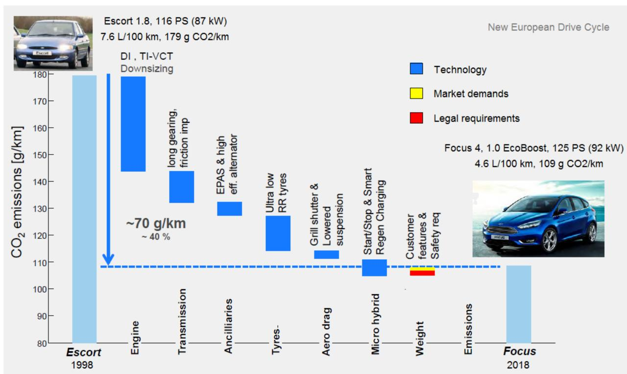
**Figure 1.** Reduction in GHG emissions through the progress in the powertrain technology over the past two decades (Source: Kramer et.al. [4]).
