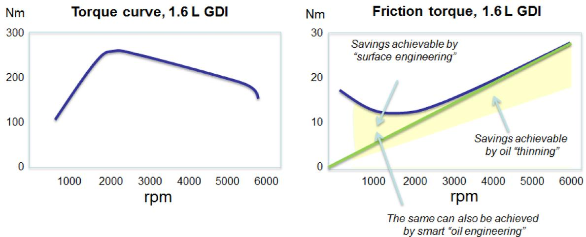
**Figure 2.** The torque curve (l.h.s.) and the friction torque (r.h.s.) for a production 1.6L i4 GDI engine. The primary engineering strategies for friction reduction are also shown [6].
