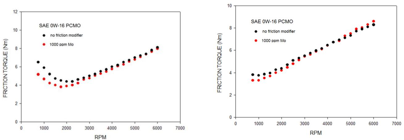
**Figure 9.** The effect of molybdenum friction modifier on engine friction: l.h.s.—Ford Duratec, r.h.s.—M.B. M133.
