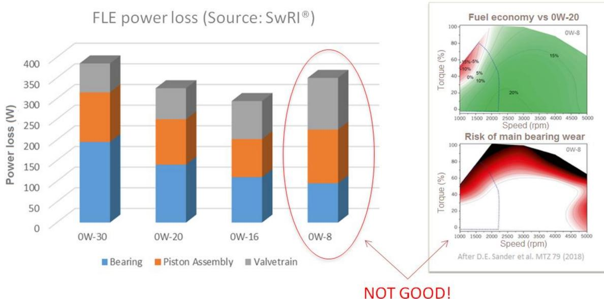
**Figure 5.** Friction power loss measured for different engine subsystems in a firing engine using different oil viscosities (l.h.s.) and simulated fuel economy and bearing health maps for SAE 0W-8 oil in a modern passenger car engine (r.h.s.).
