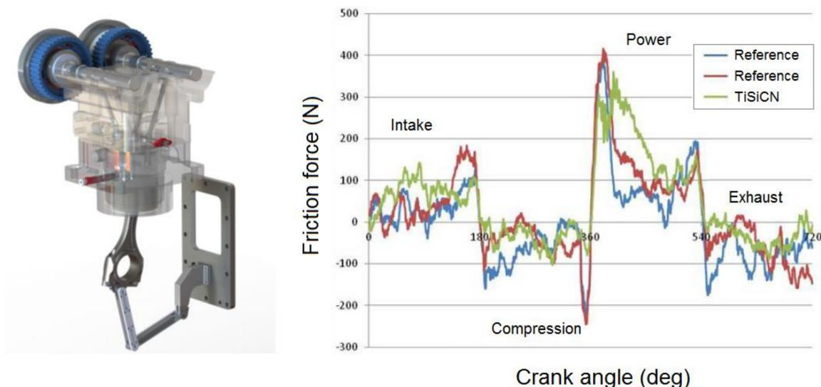
**Figure 4.** Reduction in piston/bore friction achieved on switching to TiSiCN coated top and second ring [7].
