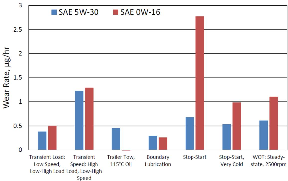
Figure 7. Liner wear rates for different engine test sequences.
