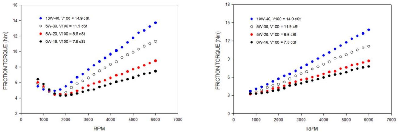
**Figure 8.** The effect of oil viscosity grade on engine friction at 90 °C: l.h.s.—Ford Duratec, r.h.s.—M.B. M133.
