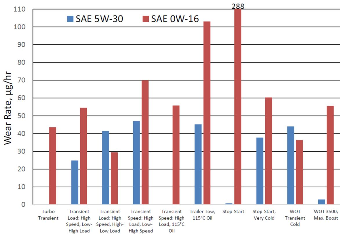
Figure 6. Top ring wear rates for different engine test sequences.
