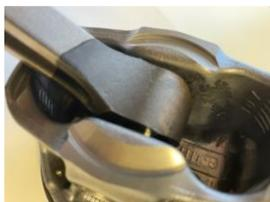
Phosphate coated bushingless small end connecting rods and DLC pins
