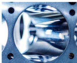
Mirror-like LDS coated cylinder bores (Daimler)
