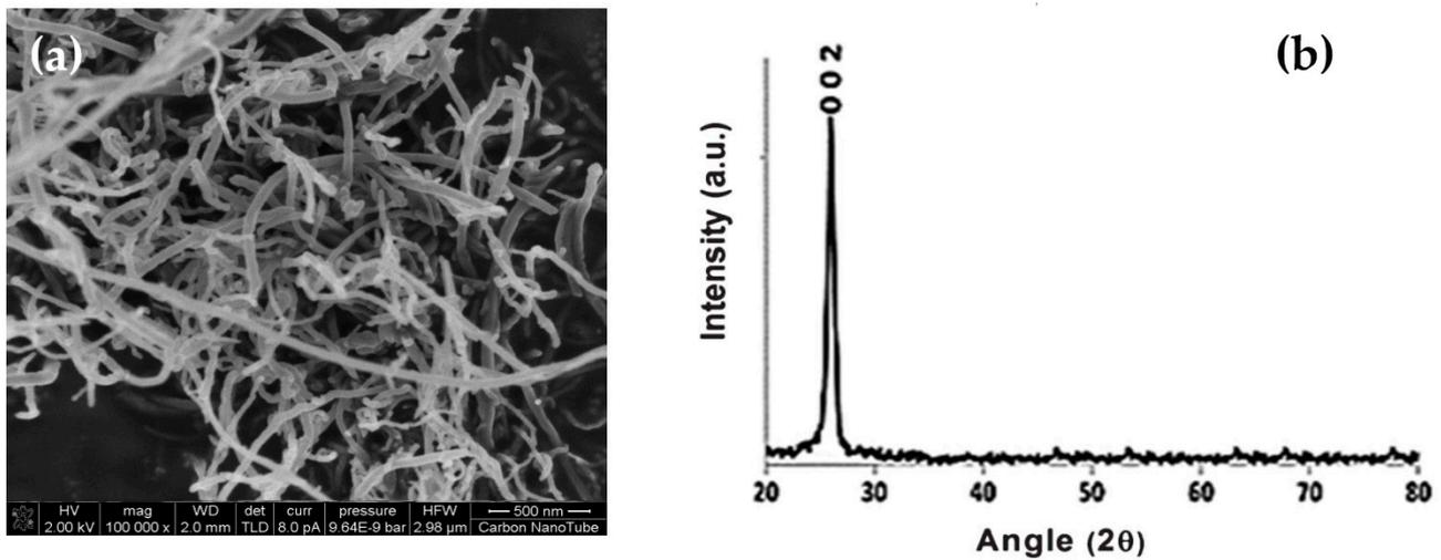
Figure 3. (a) The TEM image of the MWCNTs. (b) The XRD patterns of the MWCNTs.
