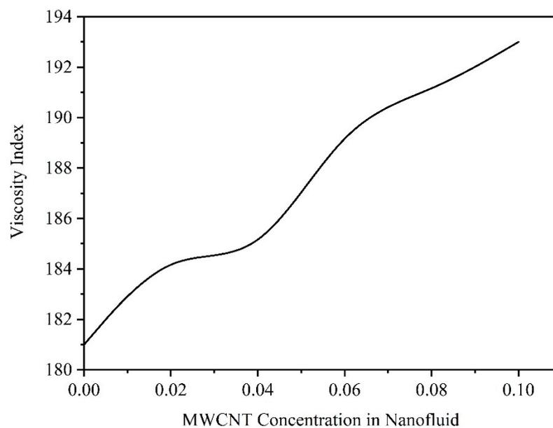
Figure 8. Viscosity index of the nanofluid vs. the CNT concentration.
