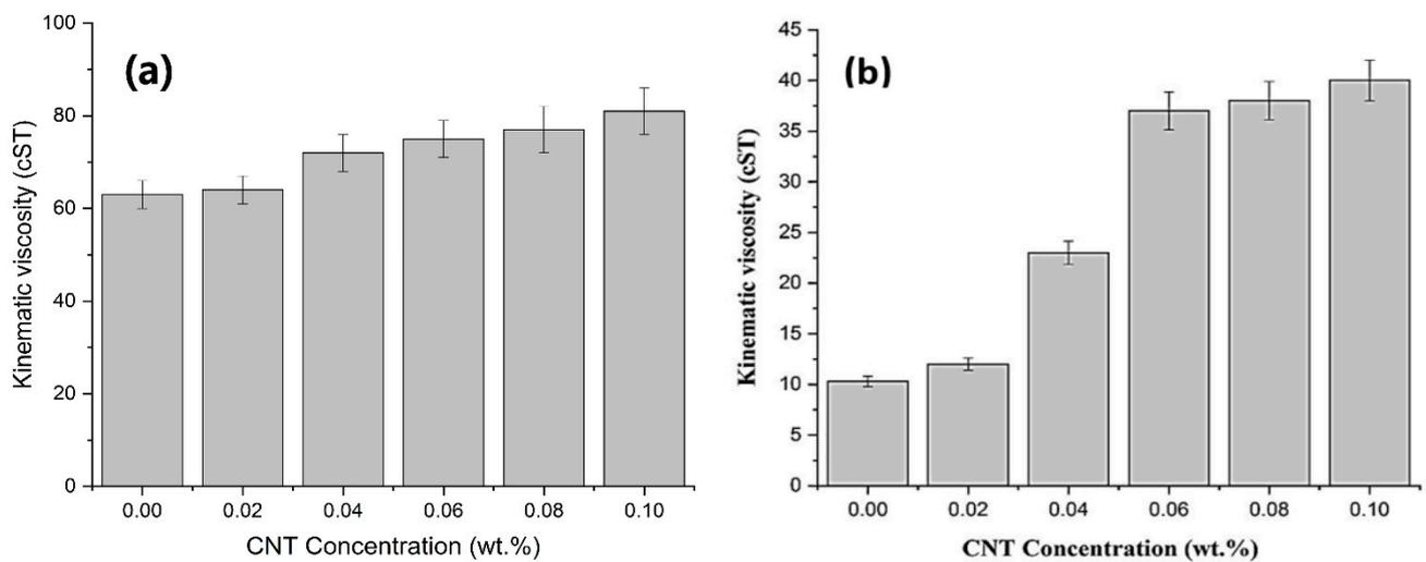
Figure 7. Kinematic viscosity of the different compositions of the nano-oil: (a) at 40 °C; (b) at 100 °C.
