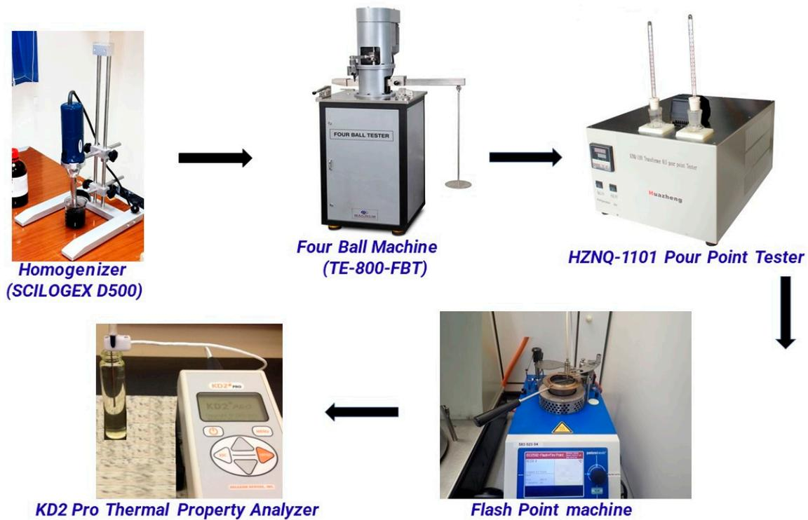
**Figure 1.** A snapshot of the equipment used for the preparation, testing, and analysis of the nano-oil.
