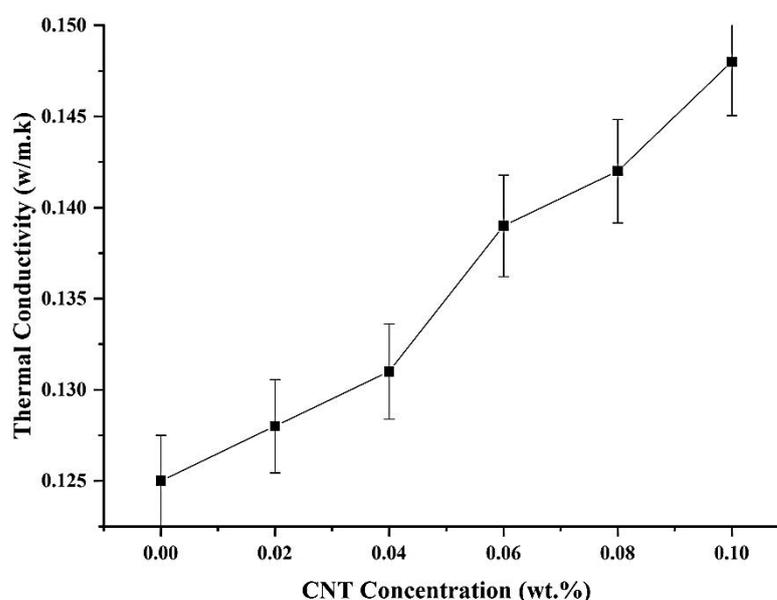
Figure 6. Thermal conductivity of the different compositions of the nano-oil.
