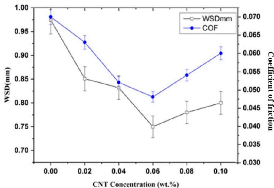
Figure 10. Friction coefficient and wear scar diameter measured for different CNTs concentrations
