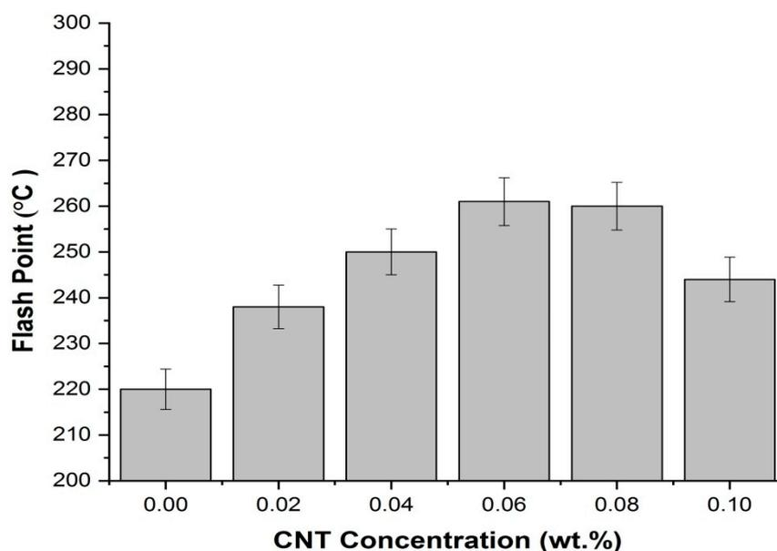
**Figure 5.** Flash point temperatures of the different compositions of the nano-oil.
