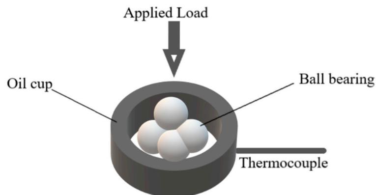
**Figure 2.** Schematic diagram of the four-ball tribo-tester.
