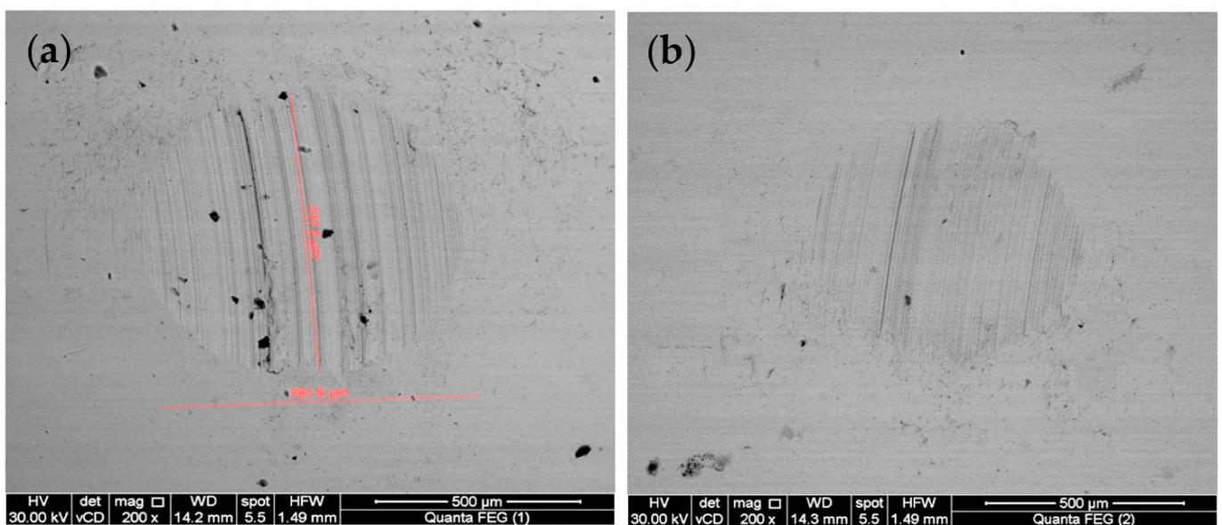
**Figure 9.** SEM of the wear scar of the steel balls lubricated by (a) SAE 5w-30 base oil; and (b) 0.06 wt.% MWCNT nano-oil.
