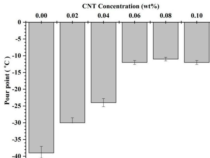
Figure 4. Pour point temperatures of the different compositions of the nano-oil.
